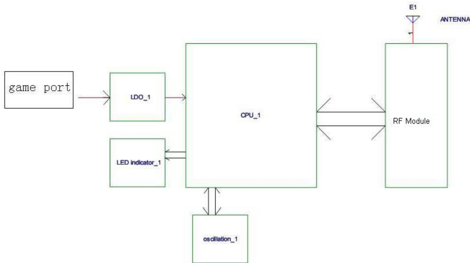
1. CPU: according the oscillation time base, receive the RF module signal and command and sent the game port command and signal to RF module. Make sure the data and signal is right to receive and sent!
