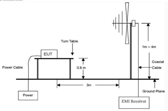
The diagram below shows the test setup that is utilized to make the measurements for emission from 1 GHz to 5 GHz Emissions.
