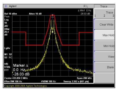
Operation frequency : 433.92 MHz Channel spacing : 25 kHz
