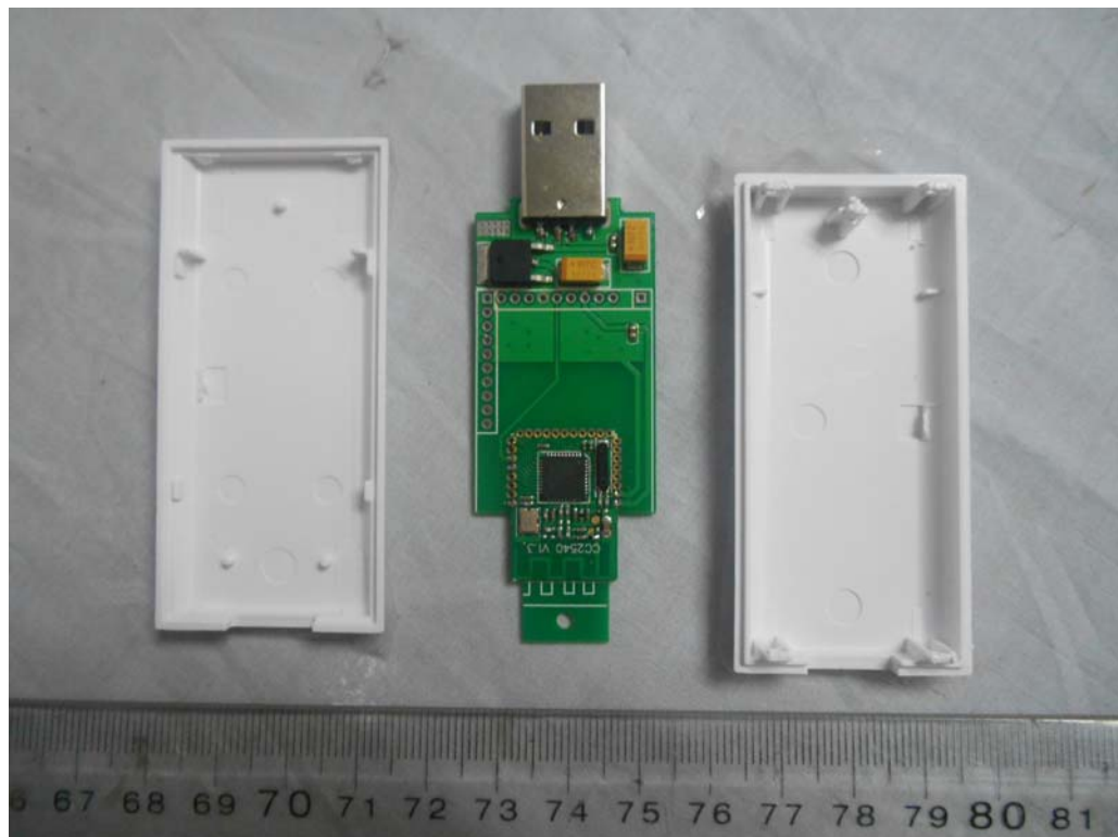
FIGURE 3 BLUETOOTH (M/N: BT-ADJUSTABLE BED) COVER REMOVED
