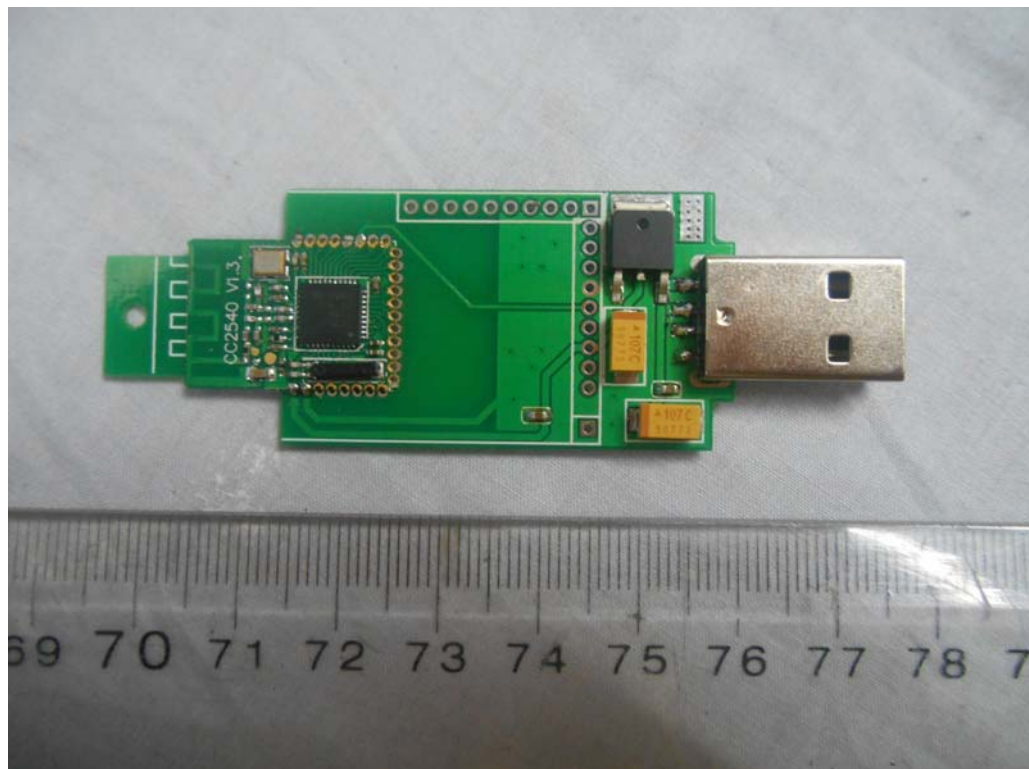
FIGURE 4 BLUETOOTH (M/N: BT-ADJUSTABLE BED) MAIN BOARD (FRONT VIEW)
