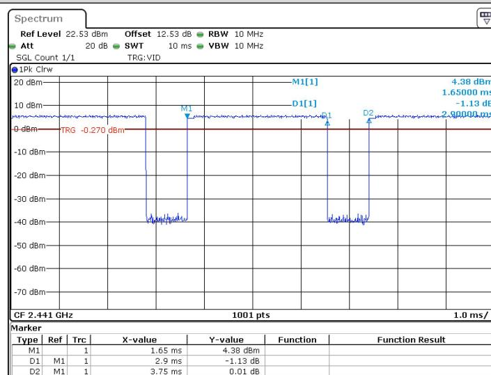
**Test Graph\_8DPSK Duty Cycle:**
