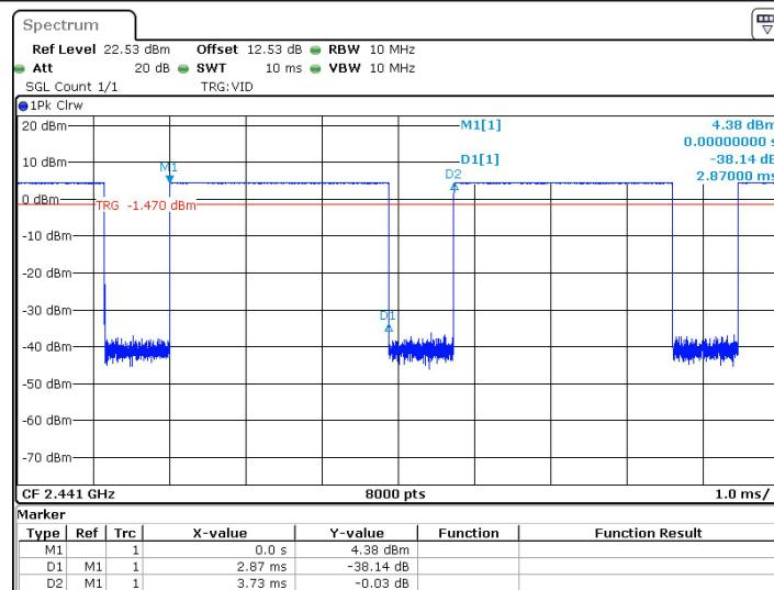
**Test Graph\_π/4DQPSK Duty Cycle:**
