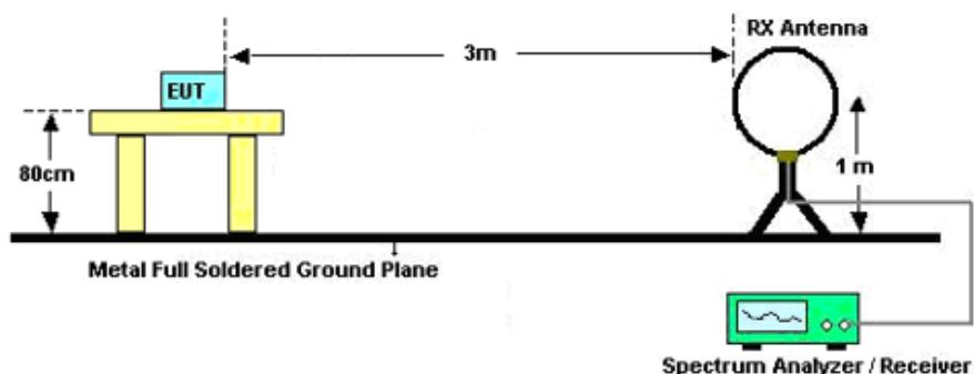
For radiated emissions from 30MHz to 1GHz
