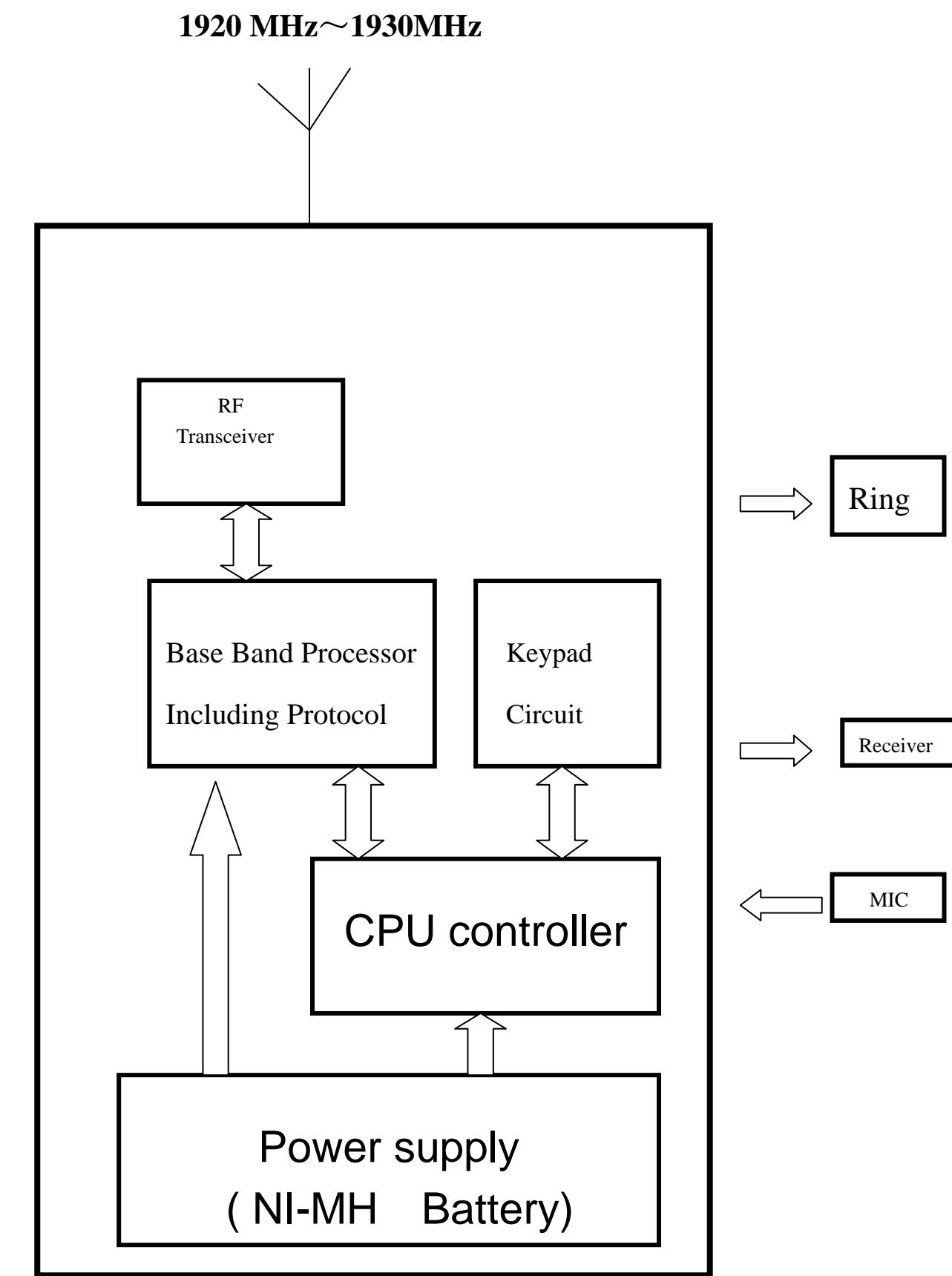
**HWD9888(48)TSD PP Block \_Diagram(Handset)**
