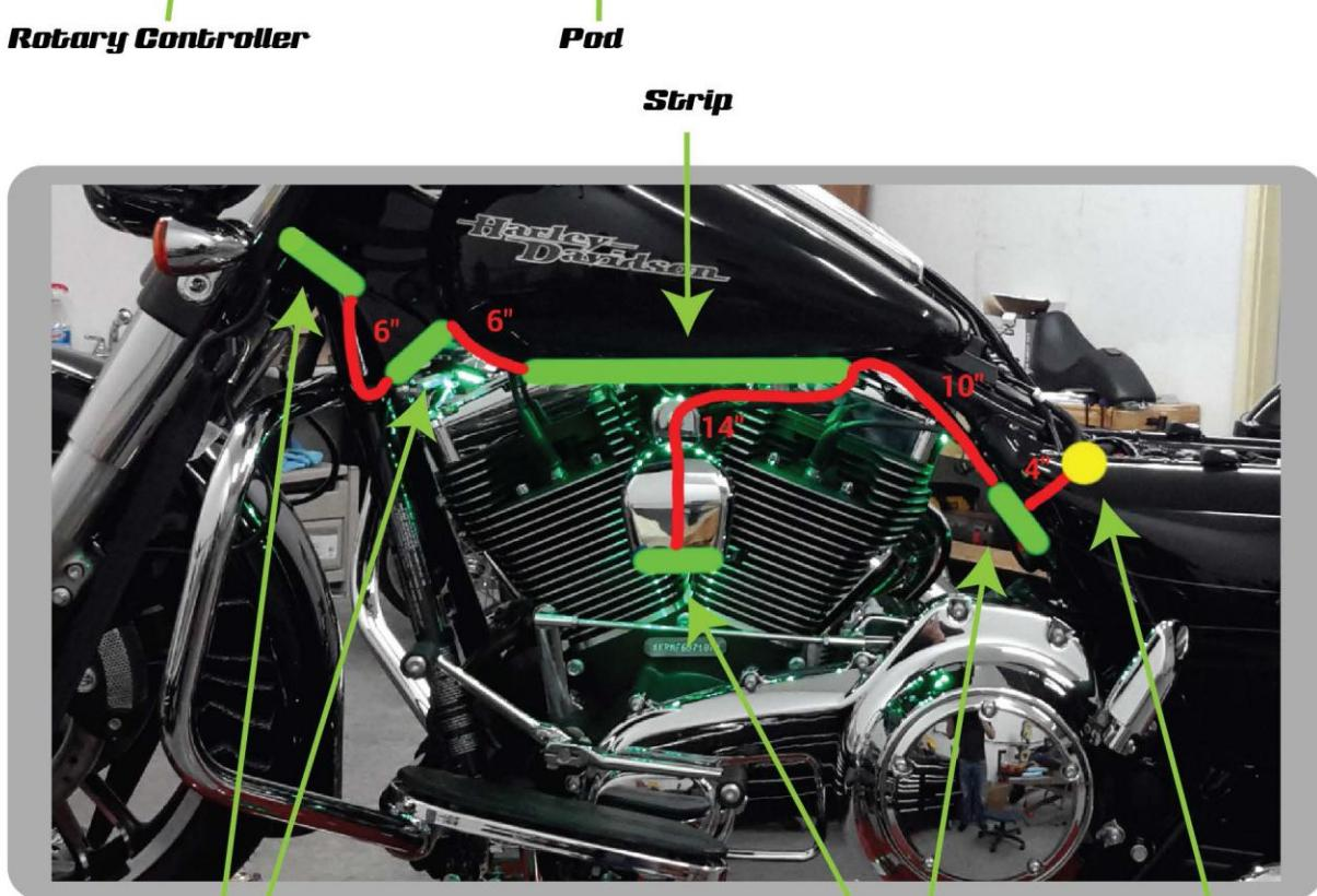
**Pictures above show the same strips and pods viewed from both sides of the motorcycle. The two pods located at the front of the motorcycle are mounted in the center.**
