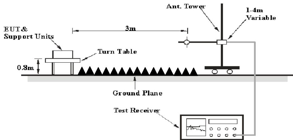
The radiated emission tests were performed in the 3 meters test site, using the setup accordance with the ANSI C63.4-2003. The specification used was the FCC 15.209, and FCC 15.247 limits.
