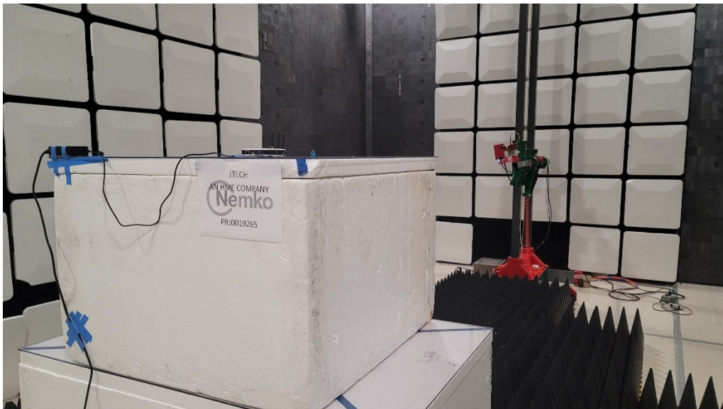
Figure 5 - Radiated emissions above 1 GHz (1 – 18 GHz), rear view.
