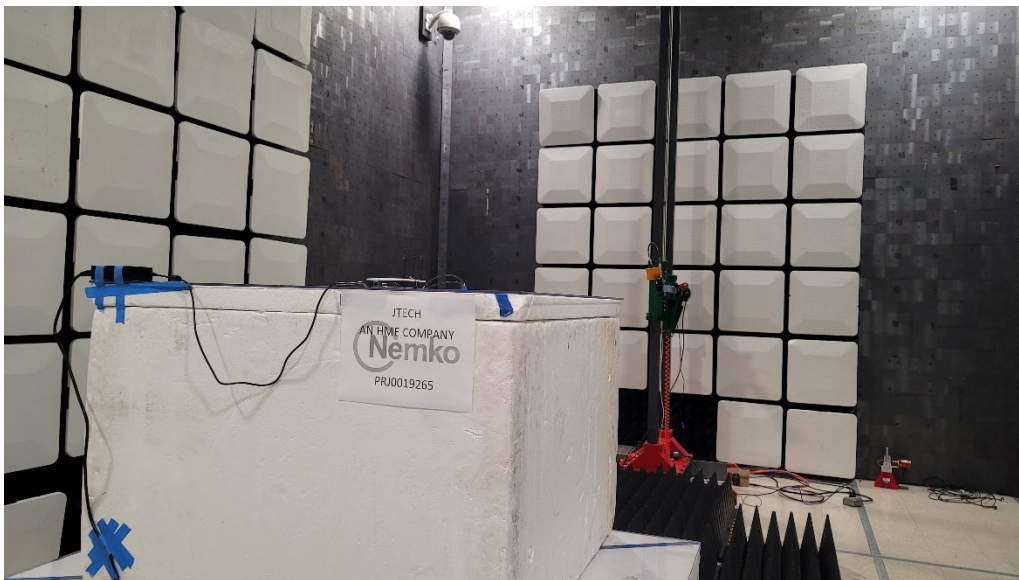
Figure 7 - Radiated emissions above 1 GHz (18 – 26 GHz).
