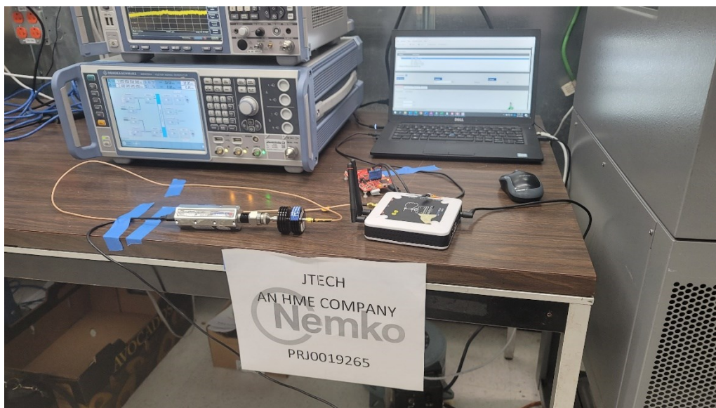
Figure 11 – Test setup: power meter, antenna conducted port.
