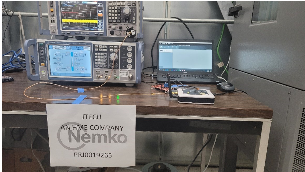
Figure 12 – Test setup: spectrum analyzer, antenna conducted port.
