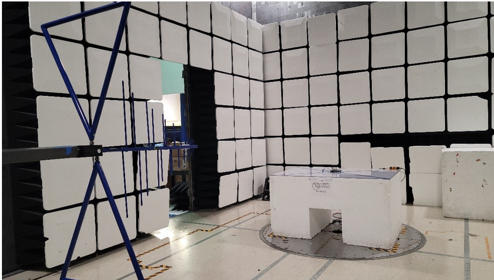
Figure 2 - Radiated emissions below 1 GHz (0.03 – 1 GHz), front view.
