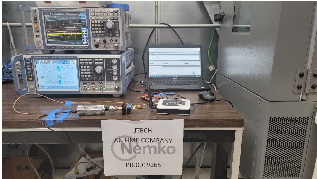
Figure 10 – Test setup: power meter, antenna conducted port.
