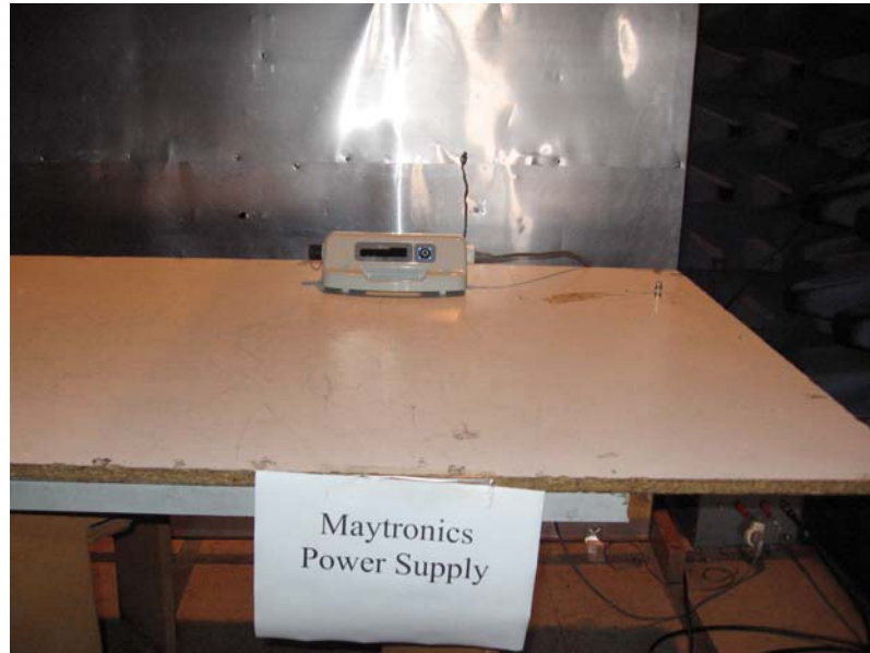
Figure 2. Conducted Emission Test
