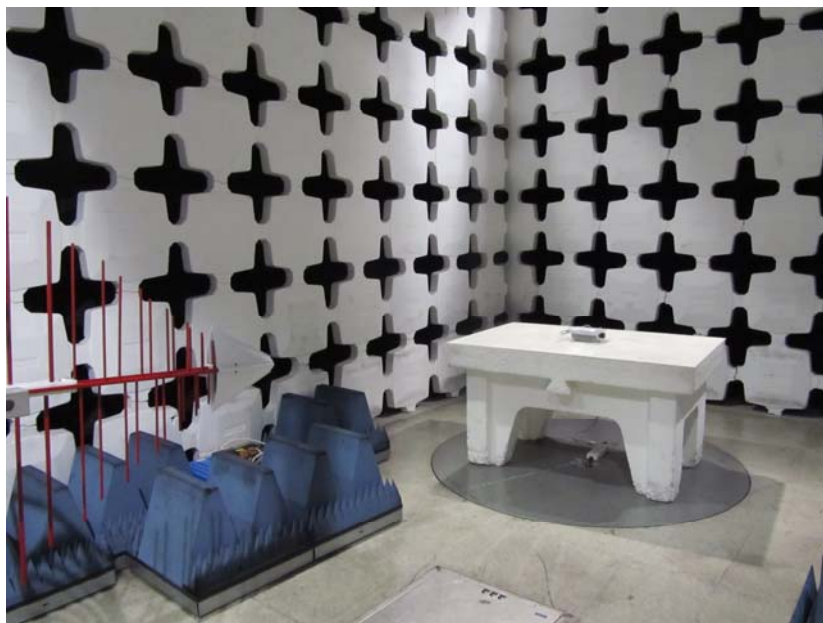
Photo 2. Radiated emissions test setup with Biconilog antenna.
