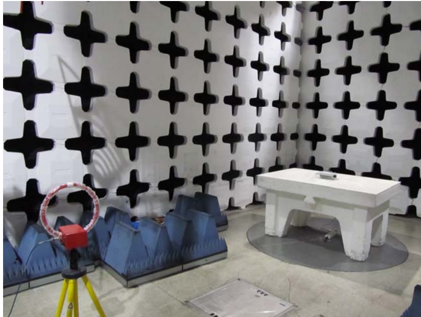
Photo 1. Radiated emissions test setup with Loop antenna.
