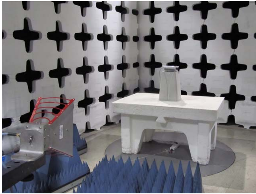
Photo 3. Radiated emissions test setup with Horn antenna in 1-18GHz.
