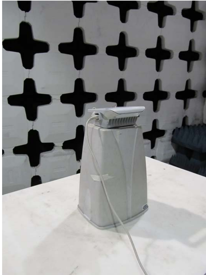
Photo 5. Radiated emissions test setup
