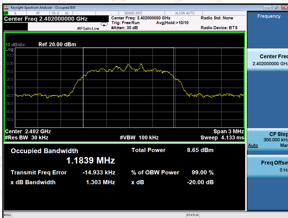
TEST PLOT OF BANDWIDTH FOR LOW CHANNEL
