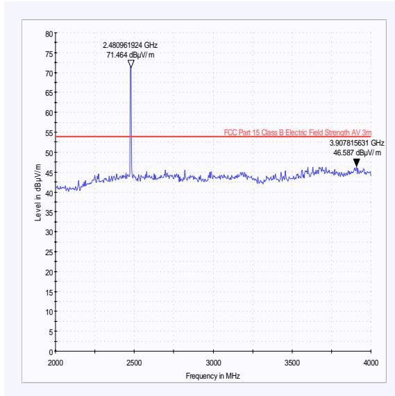
NOTE: The carrier is shown on the above plot at 2480.961 MHz
