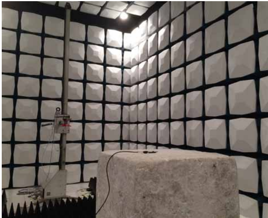
Description: Radiated Emission Test Setup for 1~18GHz
