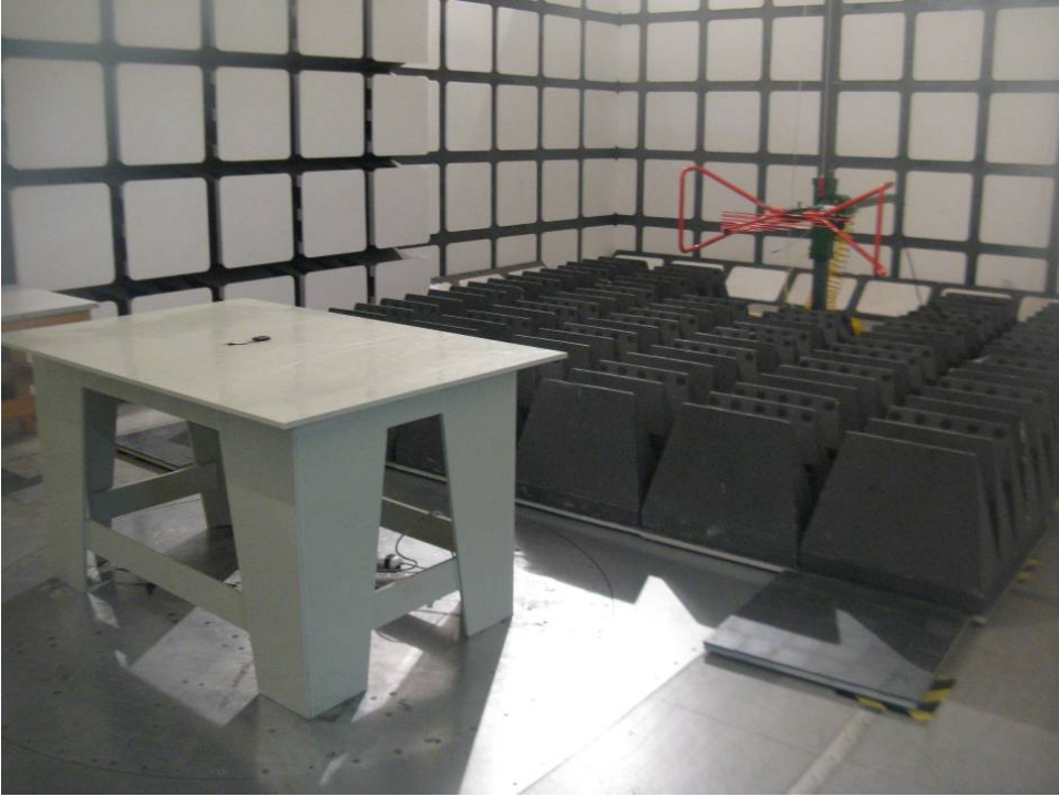
Below 1 GHz: Radiated Emissions (TX Mode) - Rear View
