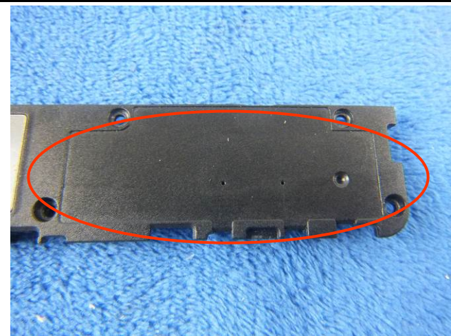
GSM/PCS/UMTS-FDD/LTE Antenna View
