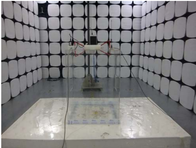
Radiated Spurious Emissions Test Setup Below 1GHz
