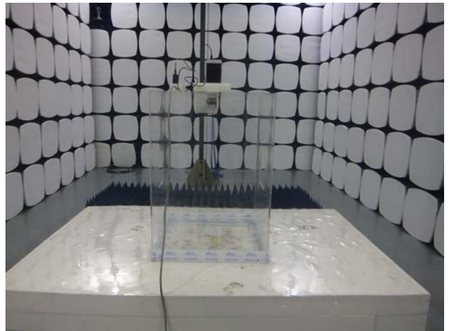
Radiated Spurious Emissions Test Setup Above 1GHz
