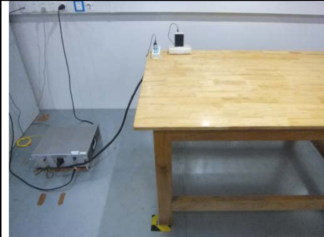
Conducted Emissions Test Setup Front View
