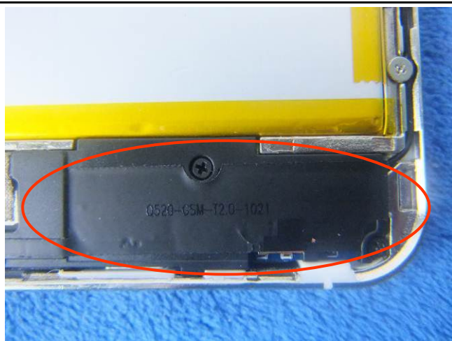
GSM/PCS/UMTS-FDD/LTE Antenna View
