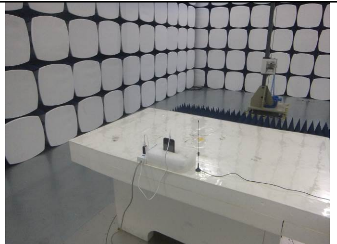
Radiated Spurious Emissions Test Setup Above 1GHz
