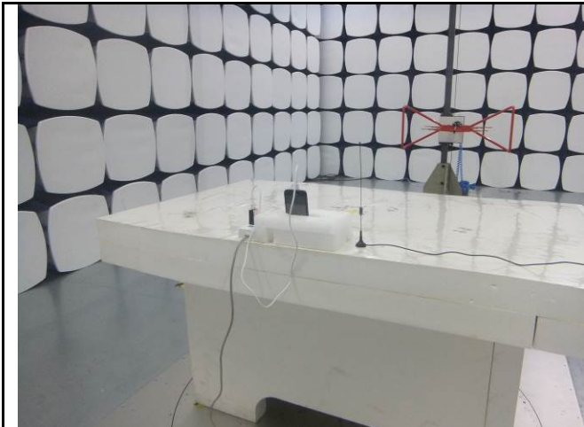
Radiated Spurious Emissions Test Setup Below 1GHz
