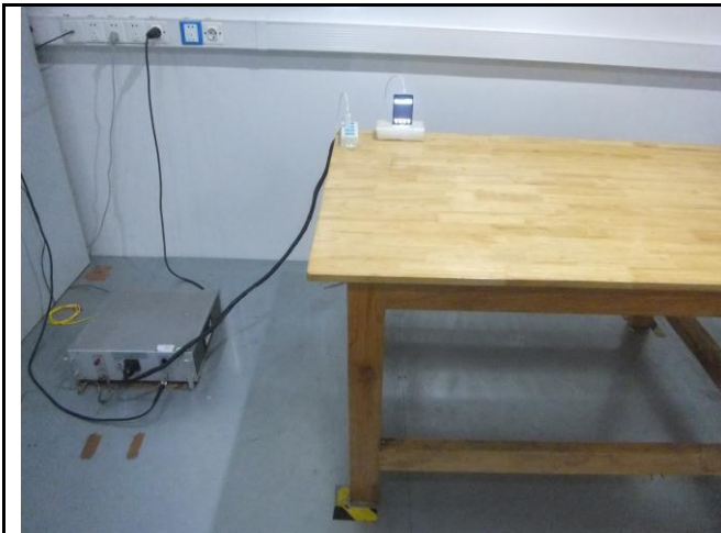
Conducted Emissions Test Setup Front View
