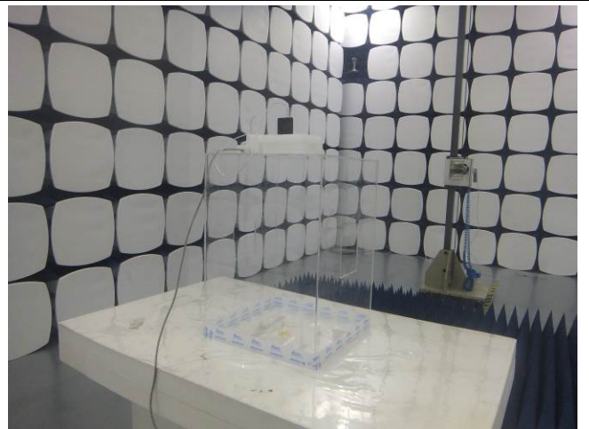
Radiated Spurious Emissions Test Setup Above 1GHz
