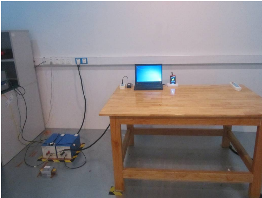
Conducted Emissions Test Setup Front View
