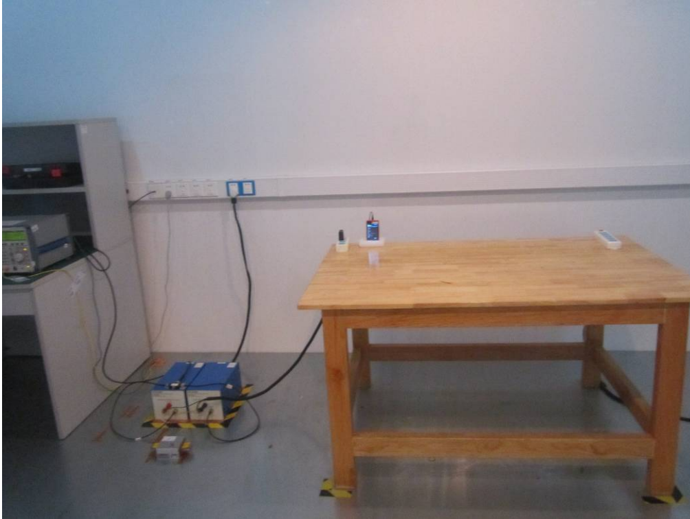
Conducted Emissions Test Setup Front View
