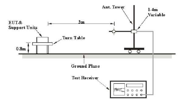
The radiated emission tests were performed in the 3 meters chamber test site, using the setup accordance with the ANSI C63.4-2009. The specification used was the FCC Part 15.109 Class B limits.
