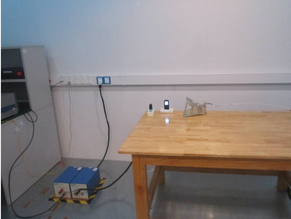
Conducted Emissions Test Setup Front View
