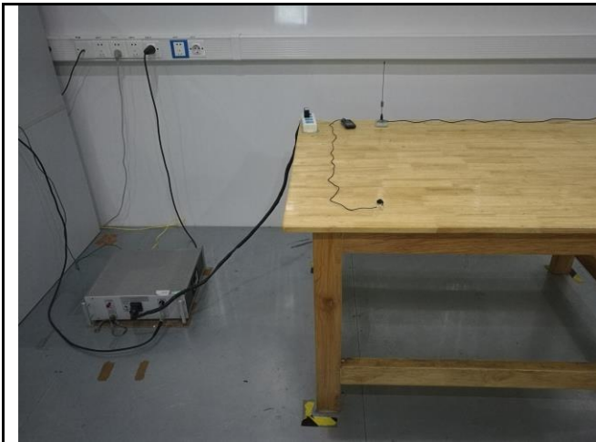
Conducted Emissions Test Setup Front View
