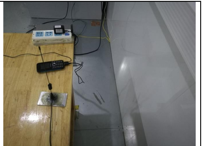
Conducted Emissions Test Setup Side View
