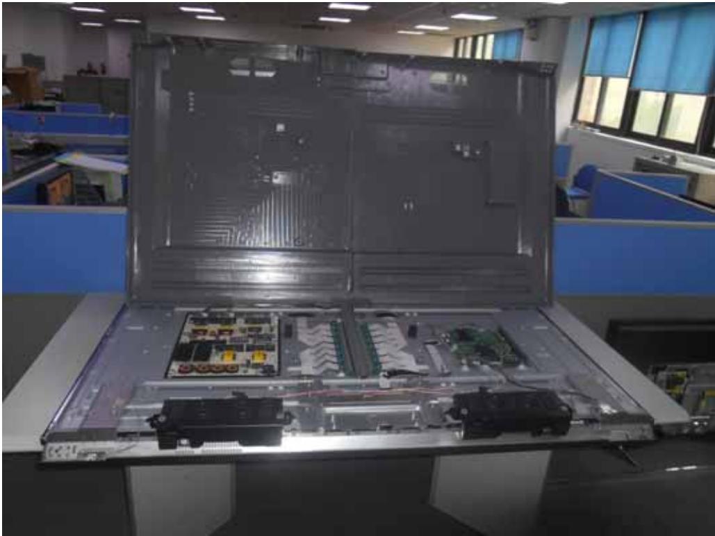
FIGURE 1 LED LCD TV (M/N: 75H10D) COVER REMOVED
