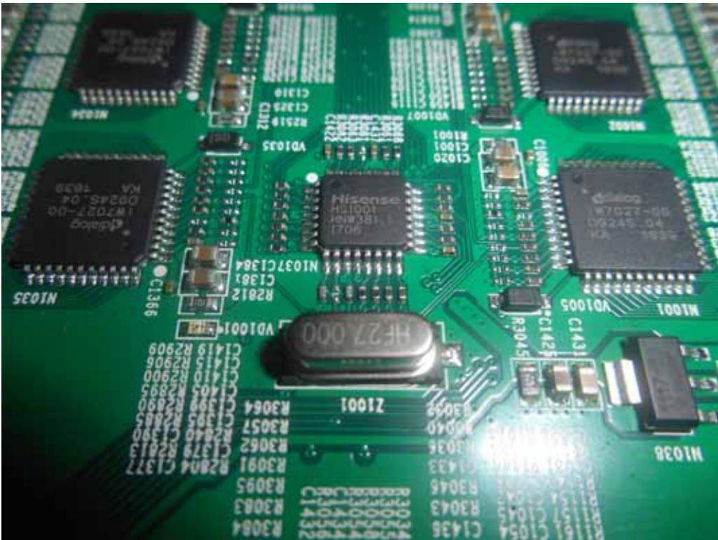
FIGURE 9 LED LCD TV (M/N: 75H10D) CHIP AND CRYSTAL ON BOARD
