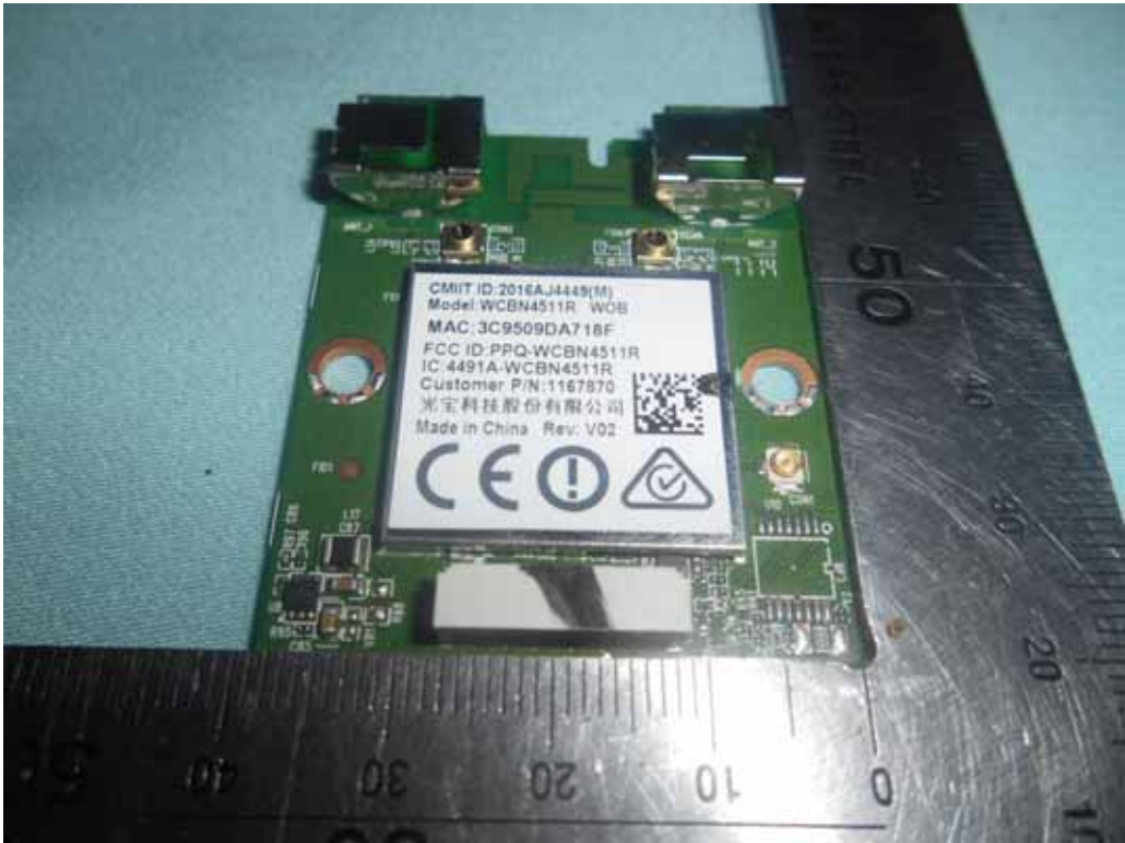
FIGURE 13 LED LCD TV (M/N: 75H10D) RF BOARD (COMPONENT SIDE)
