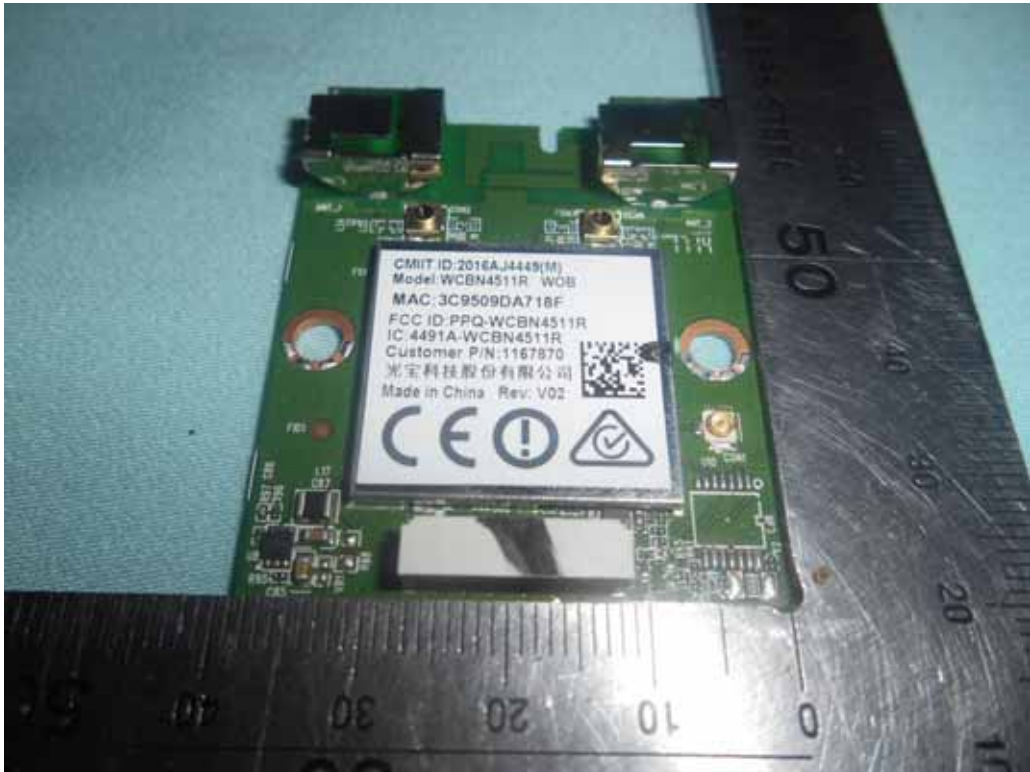
FIGURE 15 LED LCD TV (M/N: 75H10D) RF BOARD LABEL
