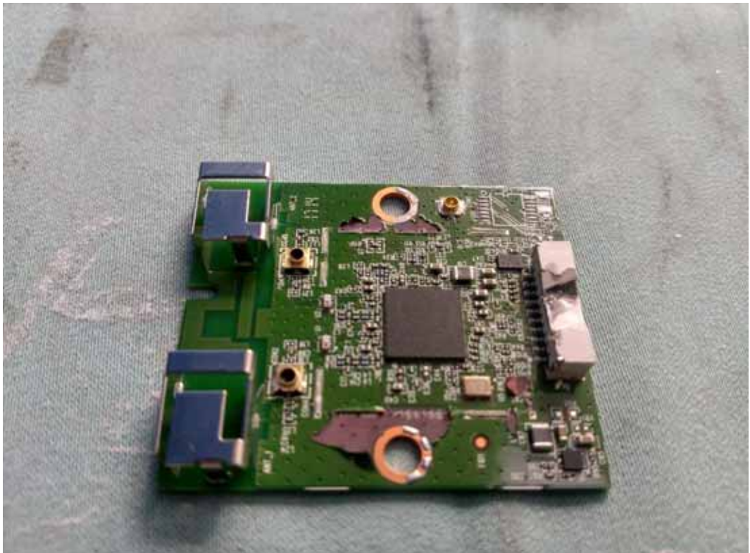
FIGURE 16 LED LCD TV (M/N: 75H10D) RF BOARD COVER REMOVED
