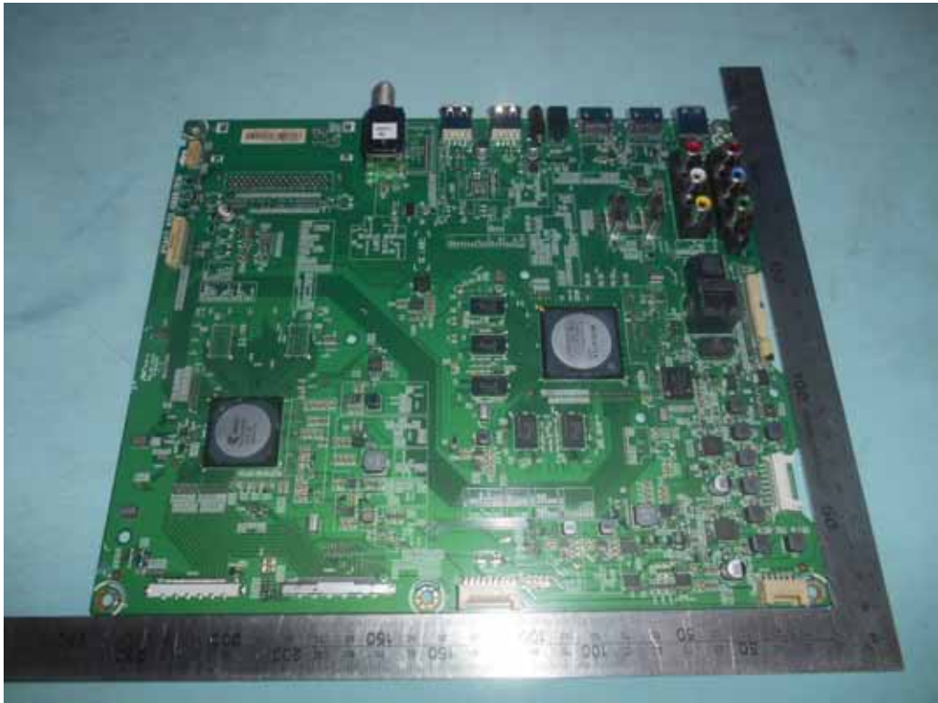
FIGURE 3 LED LCD TV (M/N: 75H10D) MAIN BOARD (COMPONENT SIDE)
