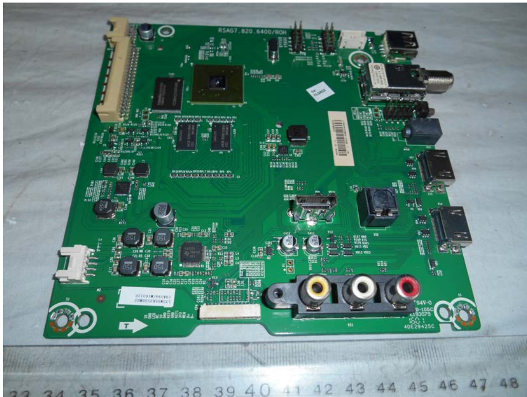
FIGURE 3 LED LCD TV (M/N: LC-55N4000U) MAIN BOARD (COMPONENT SIDE)
