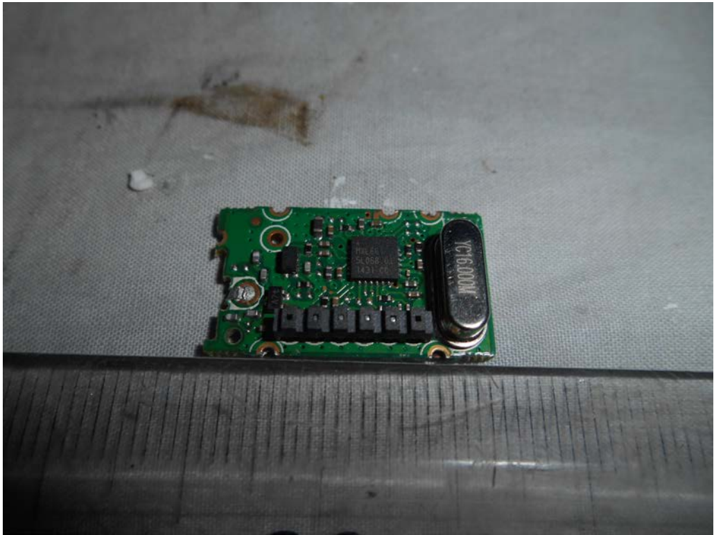
FIGURE 7 LED LCD TV (M/N: LC-55N4000U) TUNER BOARD (COMPONENT SIDE)
