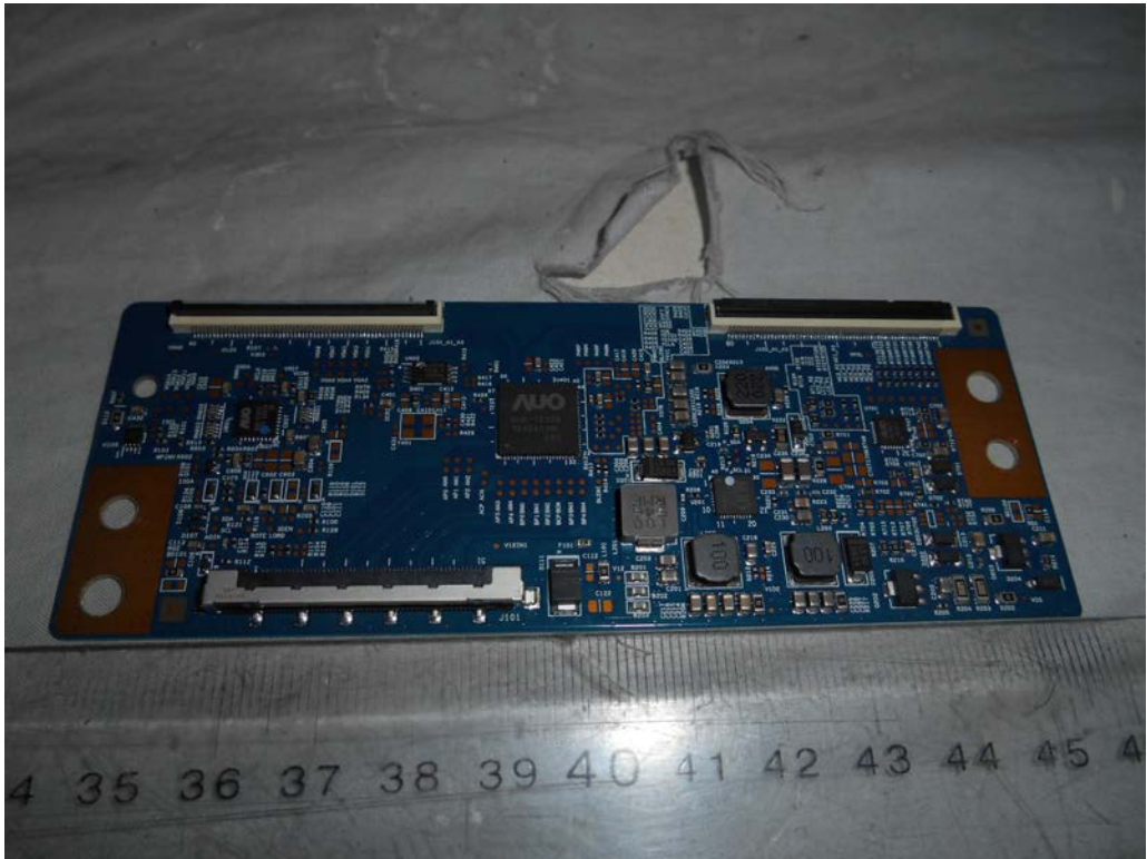
FIGURE 14 LED LCD TV (M/N: LC-55N4000U) PANEL BOARD (COMPONENT SIDE)
