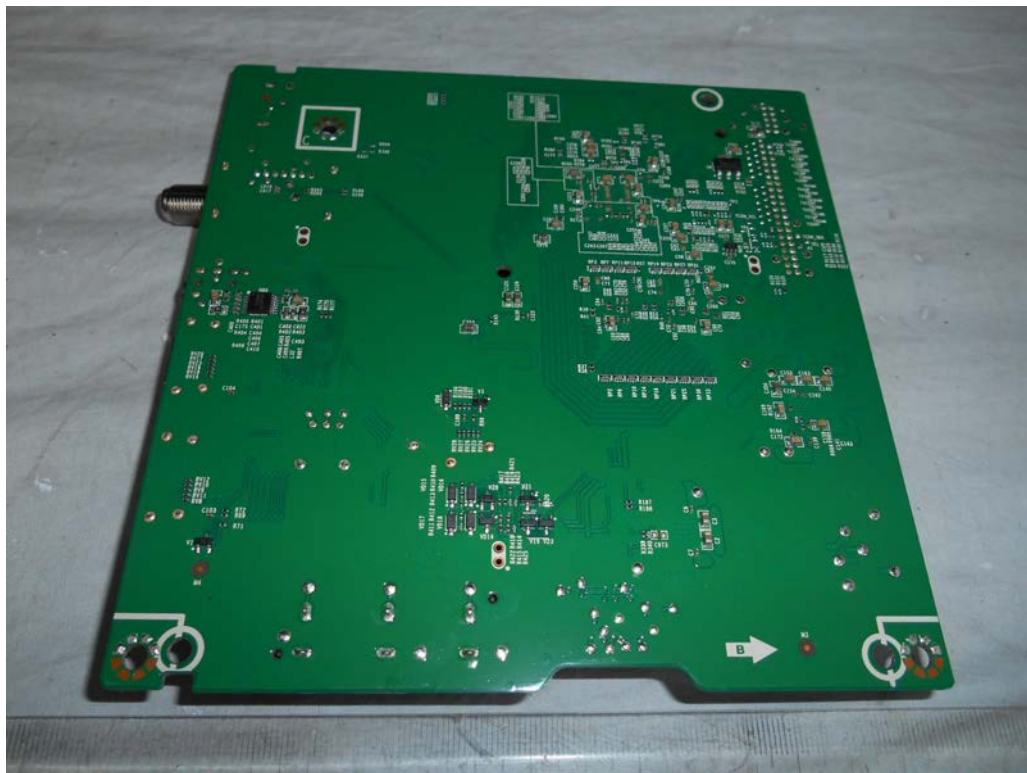
FIGURE 4 LED LCD TV (M/N: LC-55N4000U) MAIN BOARD (SOLDERED SIDE)
