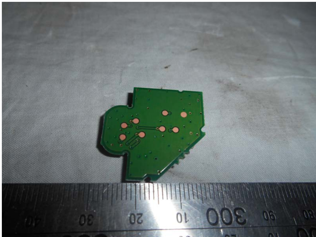
FIGURE 22 LED LCD TV (M/N: LC-55N4000U) IR BOARD (SOLDERED SIDE)
