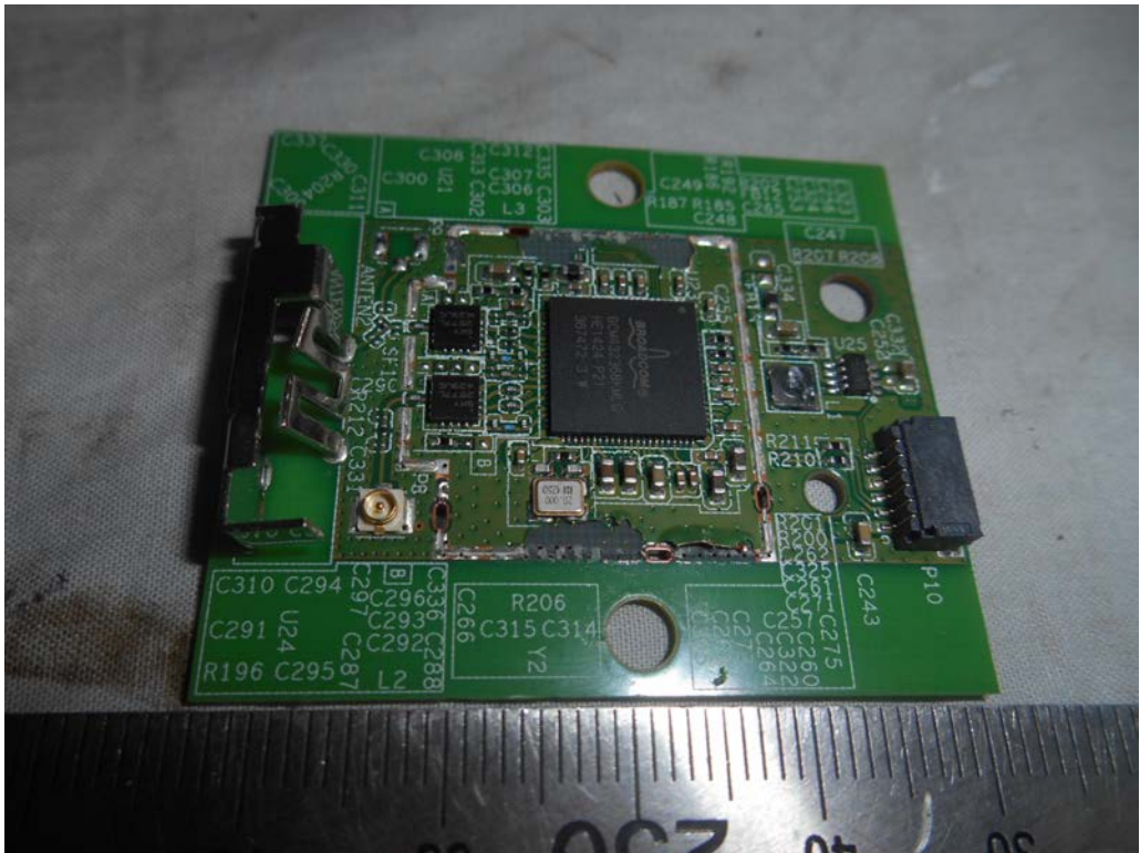
FIGURE 13 LED LCD TV (M/N: LC-55N4000U) RF BOARD COVER REMOVED
