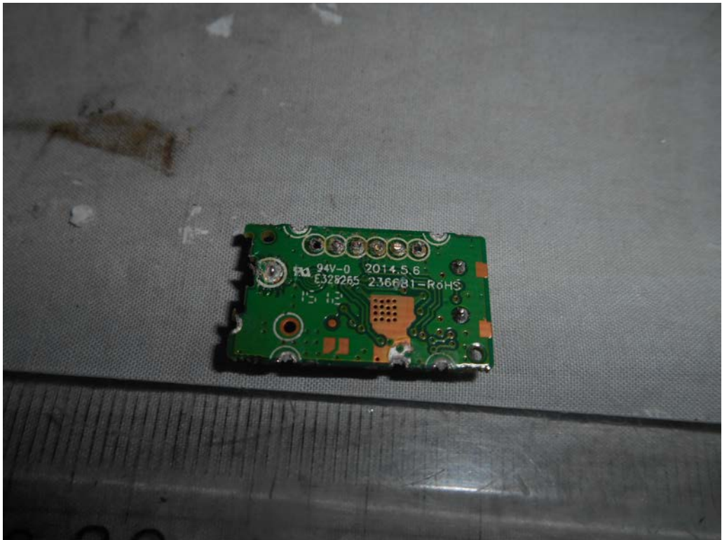
FIGURE 8 LED LCD TV (M/N: LC-55N4000U) TUNER BOARD (SOLDERED SIDE)
