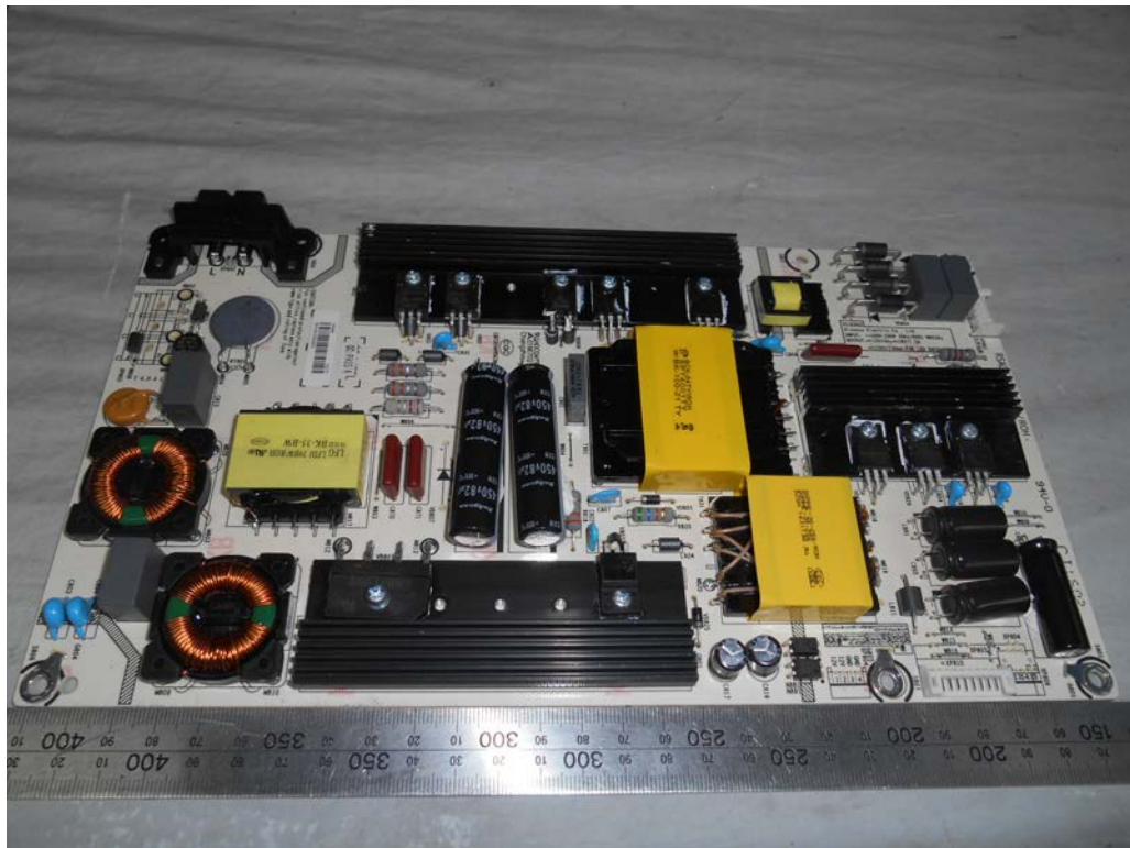
FIGURE 17 LED LCD TV (M/N: LC-55N4000U) POWER BOARD (COMPONENT SIDE)
