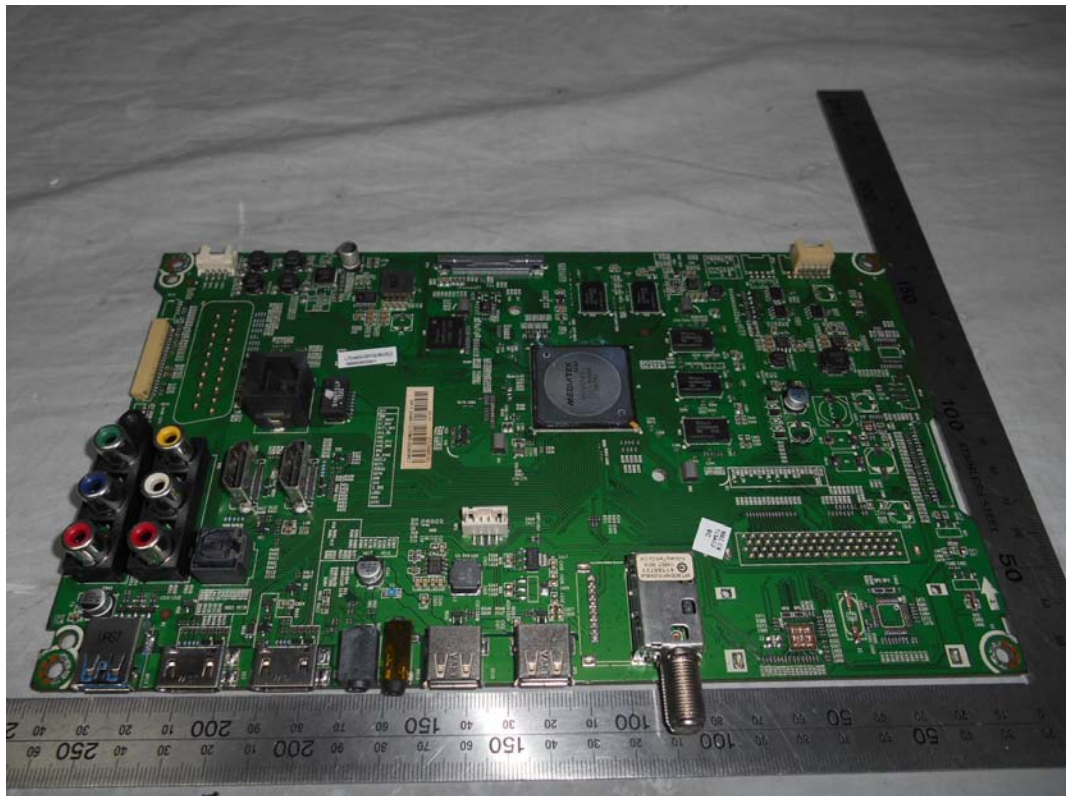
FIGURE 3 LED LCD TV (M/N: LC-50N6000U) MAIN BOARD (COMPONENT SIDE)
