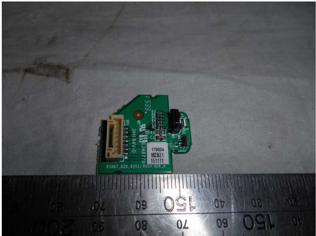
FIGURE 21 LED LCD TV (M/N: LC-50N6000U) IR BOARD (COMPONENT SIDE)
