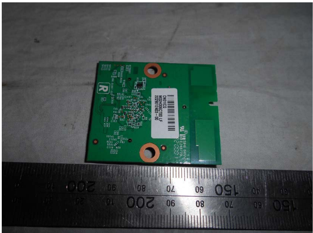
FIGURE 14 LED LCD TV (M/N: LC-50N6000U) RF BOARD (SOLDERED SIDE)
