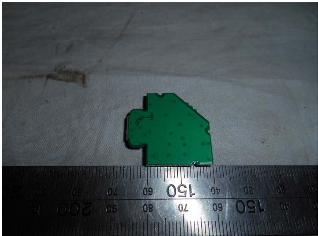
FIGURE 22 LED LCD TV (M/N: LC-50N6000U) IR BOARD (SOLDERED SIDE)
