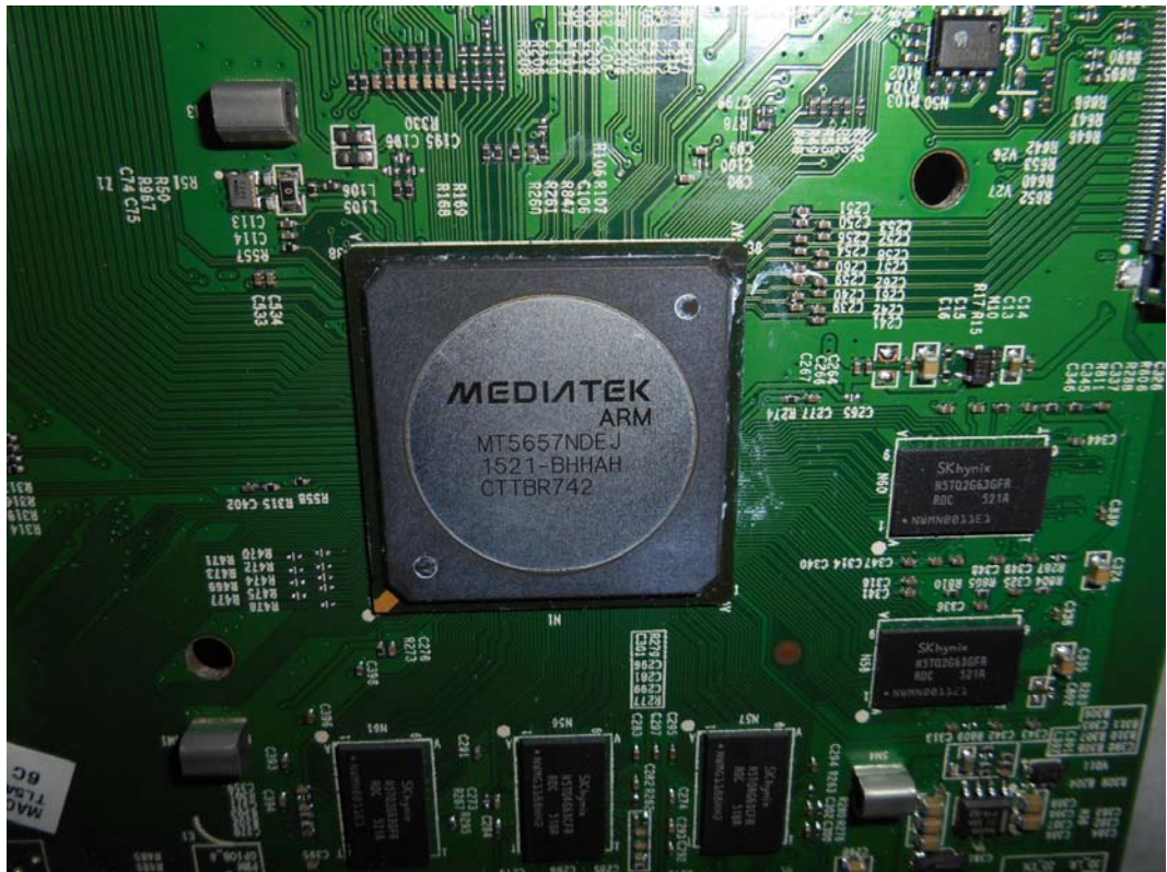
FIGURE 5 LED LCD TV (M/N: LC-50N6000U) CHIP & CRYSTAL ON MAIN BOARD
