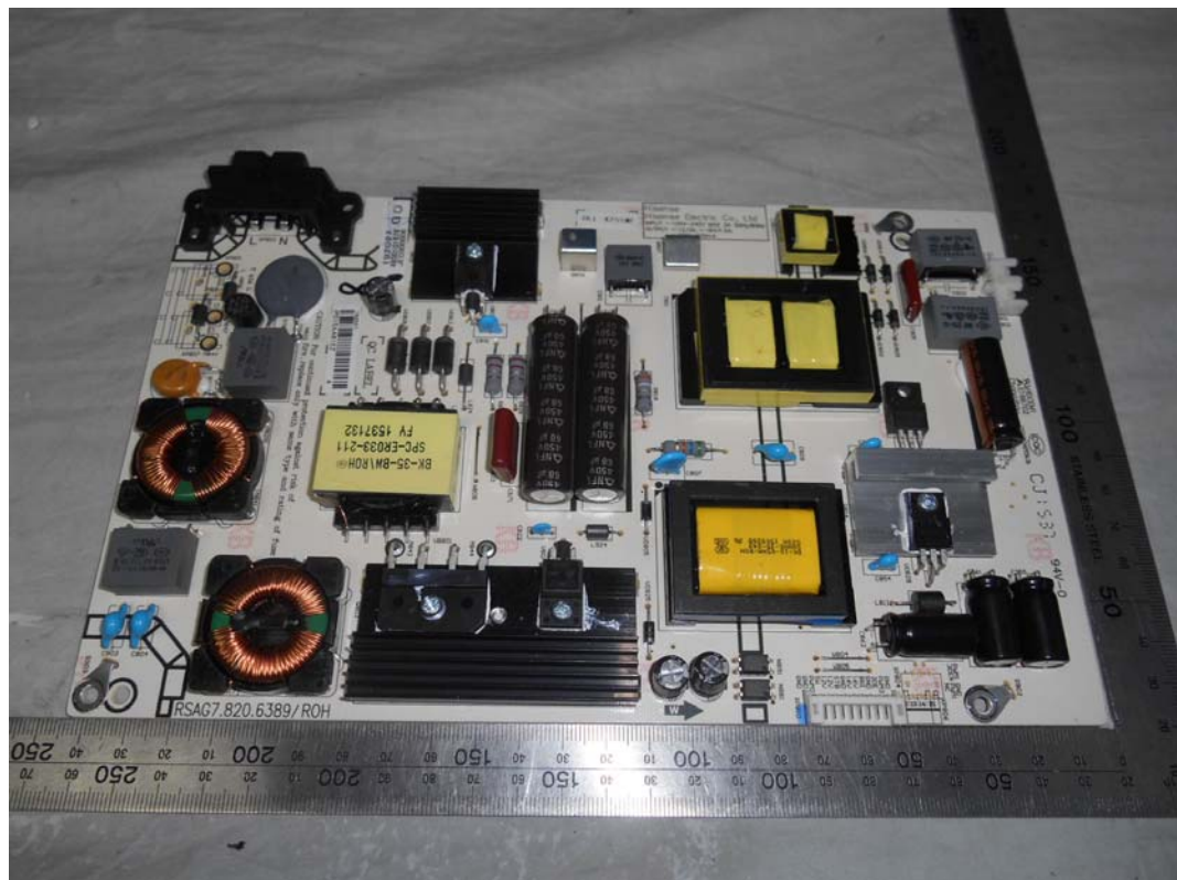
FIGURE 17 LED LCD TV (M/N: LC-50N6000U) POWER BOARD (COMPONENT SIDE)
