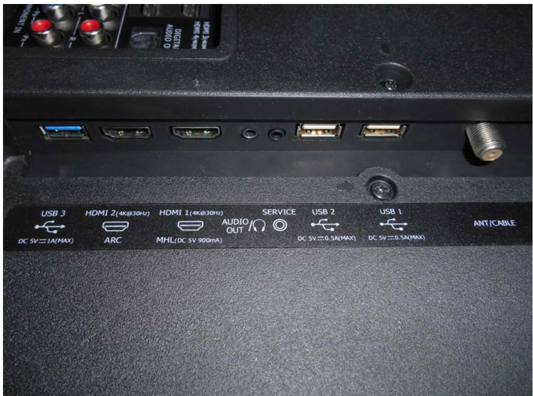
FIGURE 4 LED LCD TV (M/N: LC-50N6000U) PORTS #2
