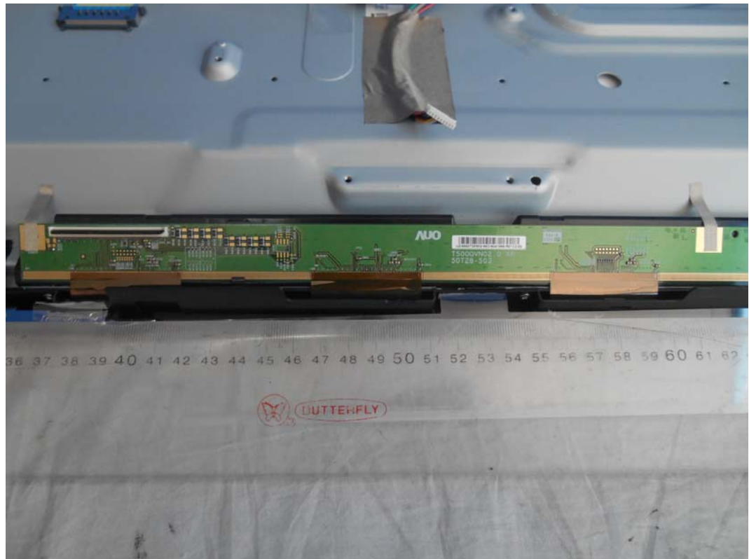
FIGURE 24 LED LCD TV (M/N: 50H7GB) CONTROL BOARD#2 (COMPONENT SIDE)
