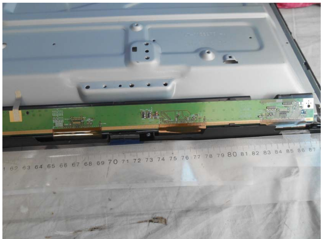
FIGURE 25 LED LCD TV (M/N: 50H7GB) CONTROL BOARD#2 (SOLDERED SIDE)
