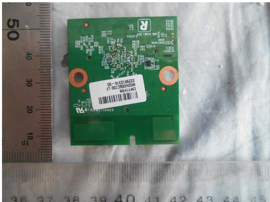
FIGURE 15 LED LCD TV (M/N: 50H7GB) RF BOARD (SOLDERED SIDE)
