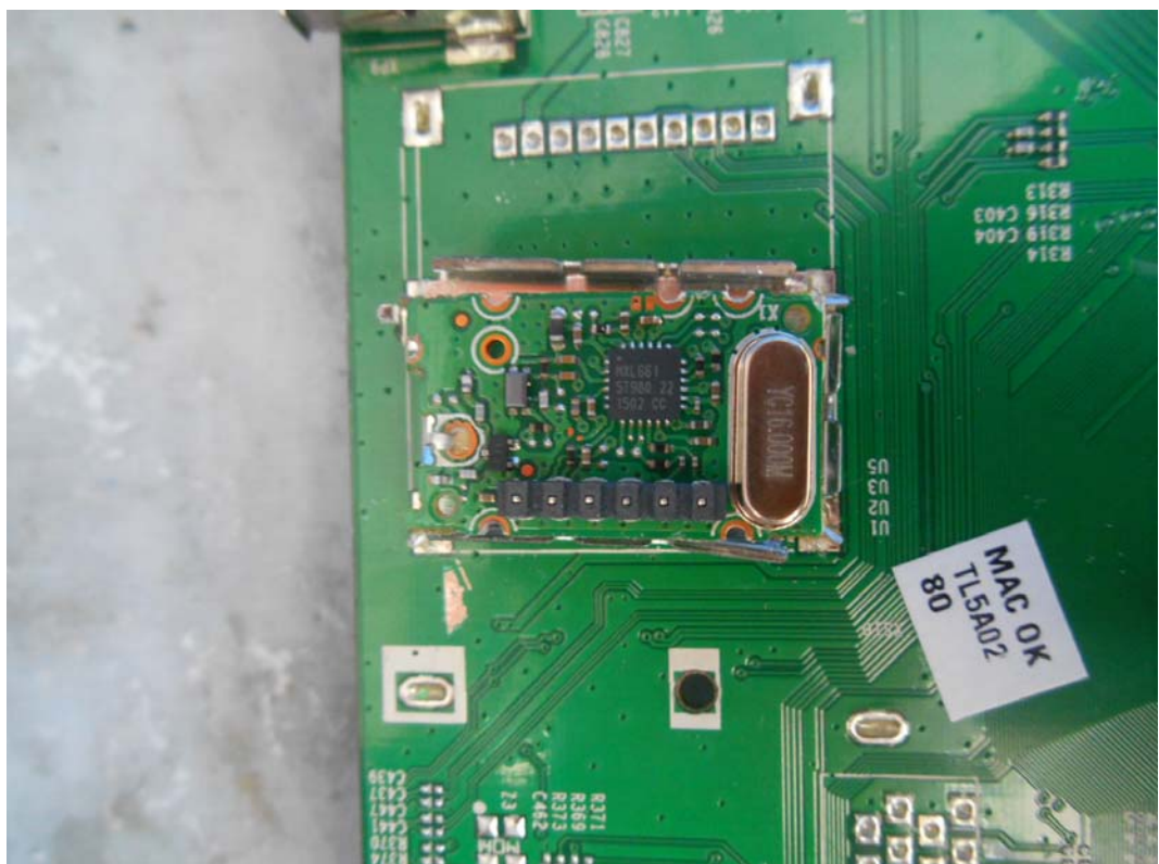
FIGURE 10 LED LCD TV (M/N: 50H7GB) TUNER ON MAIN BOARD
