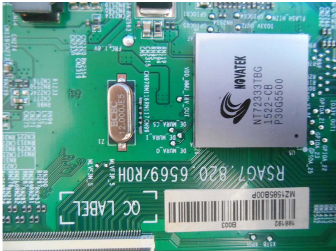
FIGURE 13 LED LCD TV (M/N: 50H7GB) CHIP AND CRYSTAL ON SIGNAL BOARD
