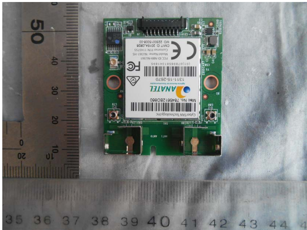
FIGURE 14 LED LCD TV (M/N: 50H7GB) RF BOARD (COMPONENT SIDE)
