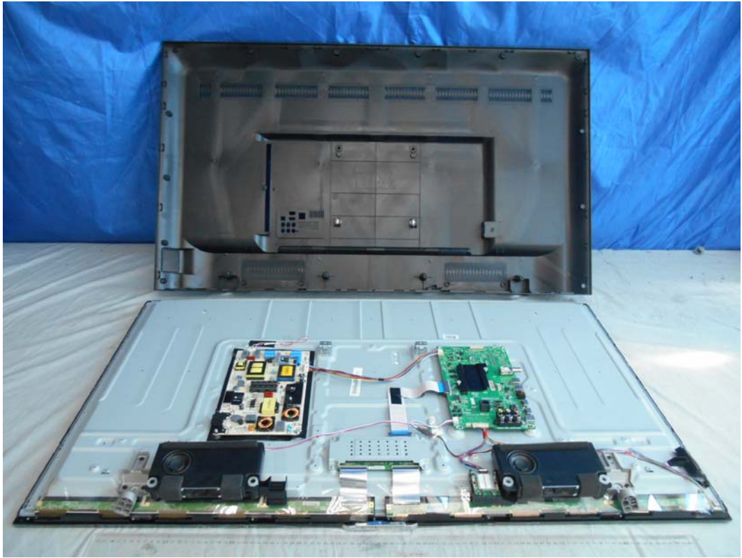
FIGURE 1 LED LCD TV (M/N: LTDN50K3201GUWUS) COVER REMOVED
