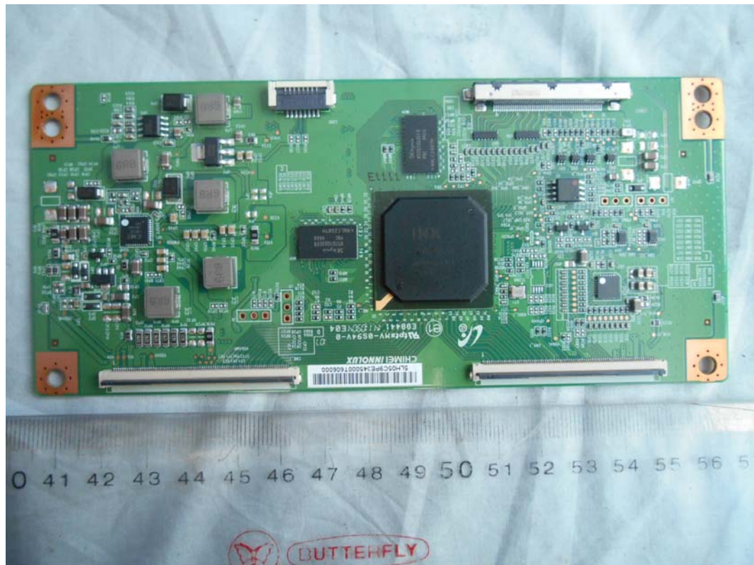
FIGURE 16 LED LCD TV (M/N: LTDN50K3201GUWUS) SIGNAL BOARD (COMPONENT SIDE)
