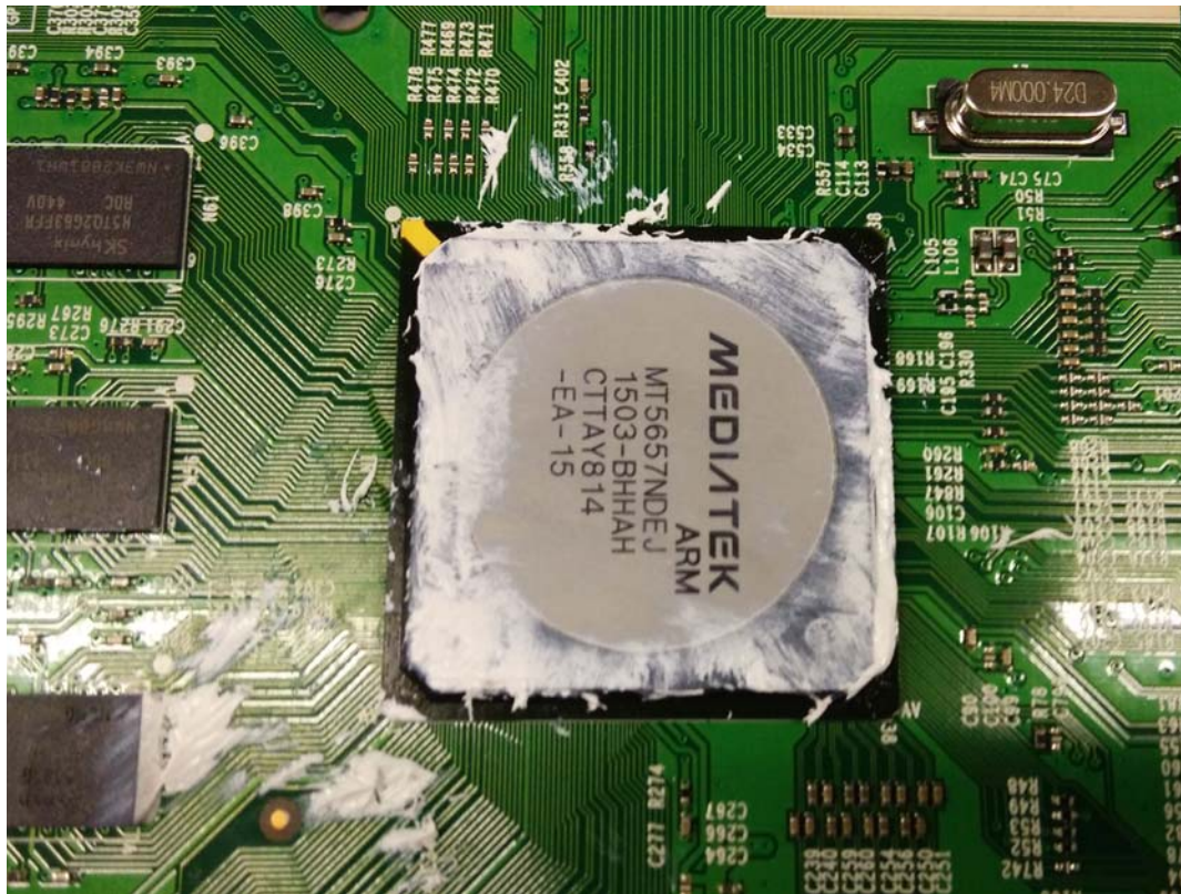
FIGURE 6 LED LCD TV (M/N: LTDN50K3201GUWUS) CHIP AND CRYSTAL ON MAIN BOARD
