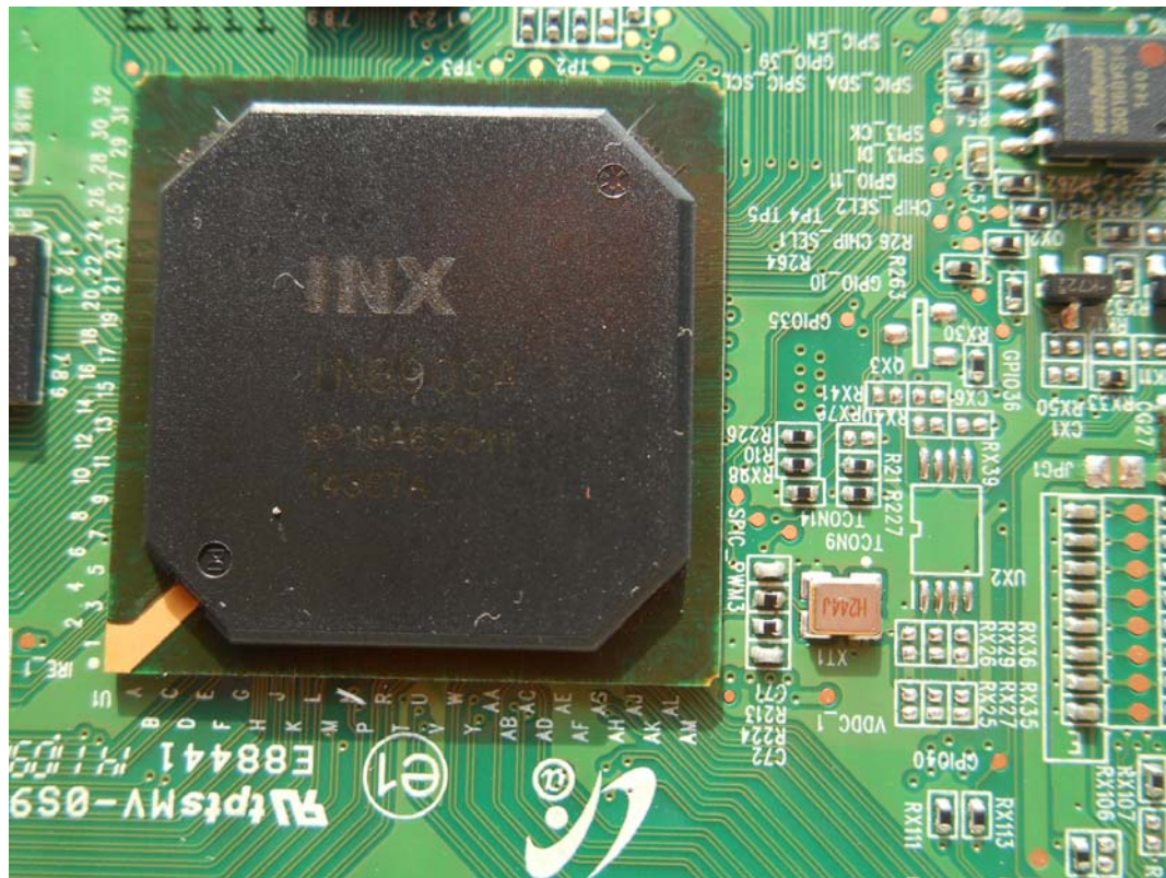
FIGURE 18 LED LCD TV (M/N: LTDN50K3201GUWUS) CHIP AND CRYSTAL ON SIGNAL BOARD
