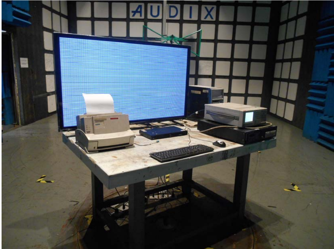
SETUP WITH MAXIMUM DETECTED EMISSION AT HORIZONTAL POLARIZATION (TEST MODE: HDMI 1280*1024@75Hz & 1kHz PLAYING)
