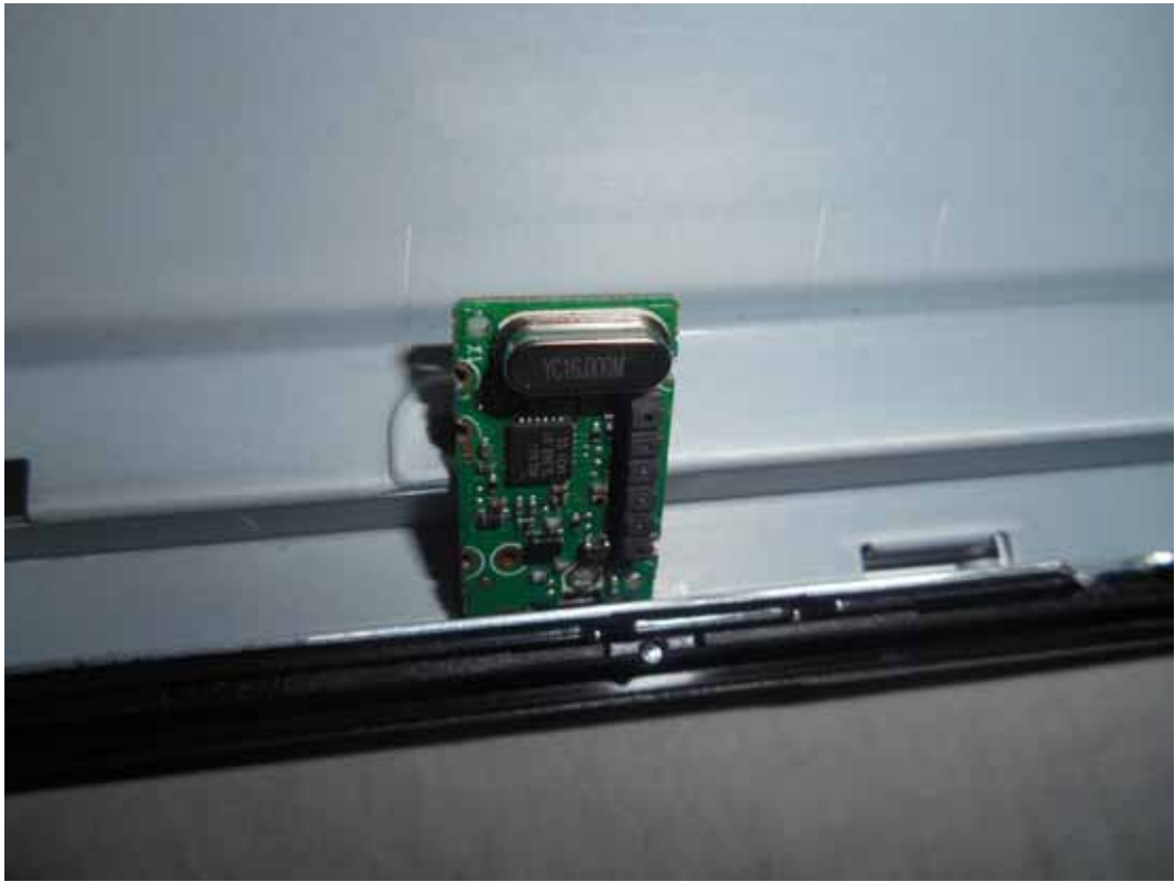
FIGURE 11 LED LCD TV (M/N: 48H4C) CHIP & CRYSTAL ON TUNER BOARD
