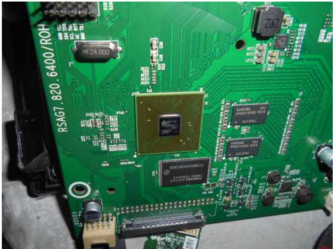
FIGURE 7 LED LCD TV (M/N: 48H4C) CHIP & CRYSTAL ON MAIN BOARD
