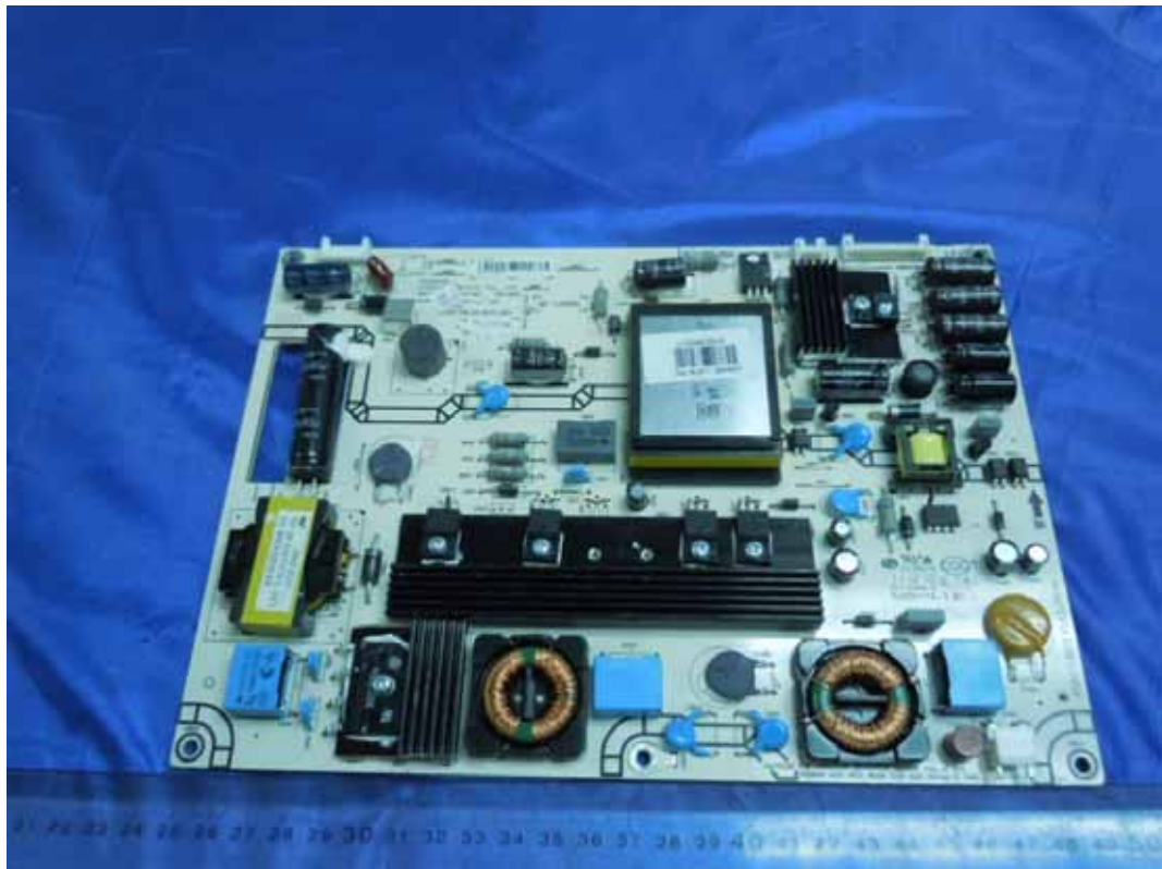
FIGURE 2 LED LCD TV (M/N: LTDN46K20US) POWER BOARD (COMPONENT SIDE)
