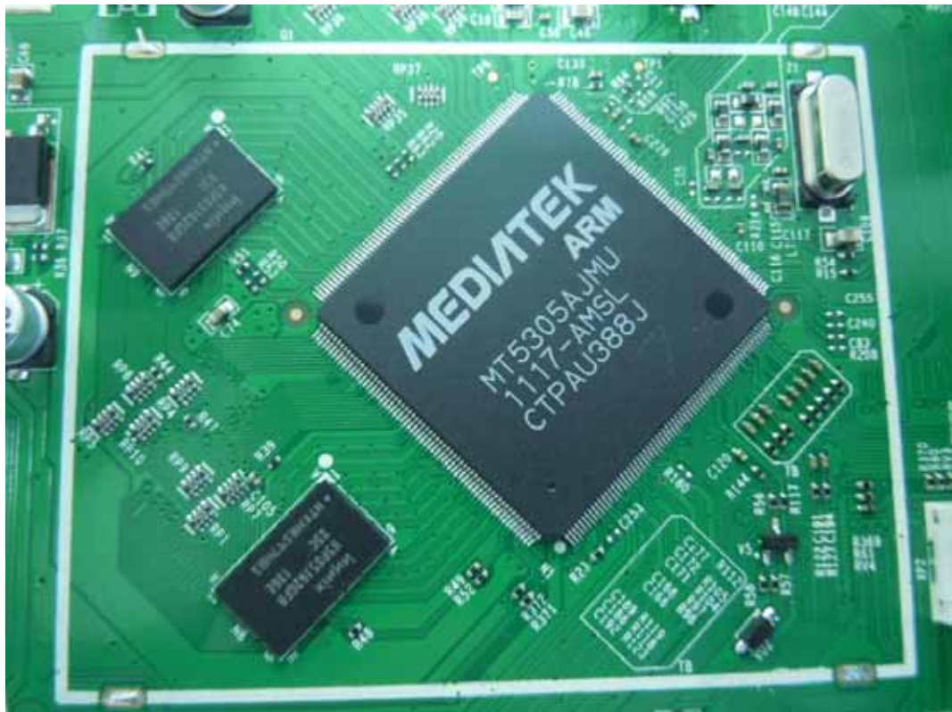
FIGURE 8 LED LCD TV (M/N: LTDN46K20US) CHIP ON MAIN BOARD
