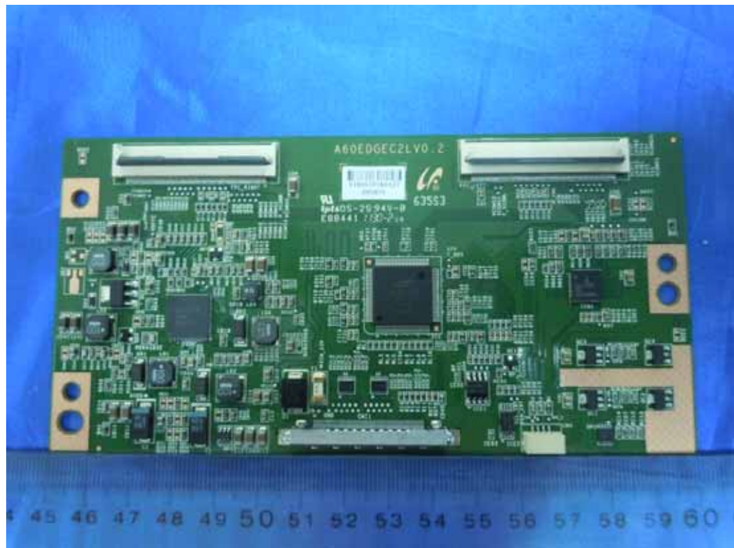
FIGURE 13 LED LCD TV (M/N: LTDN46K20US) PANEL BOARD (COMPONENT SIDE)
