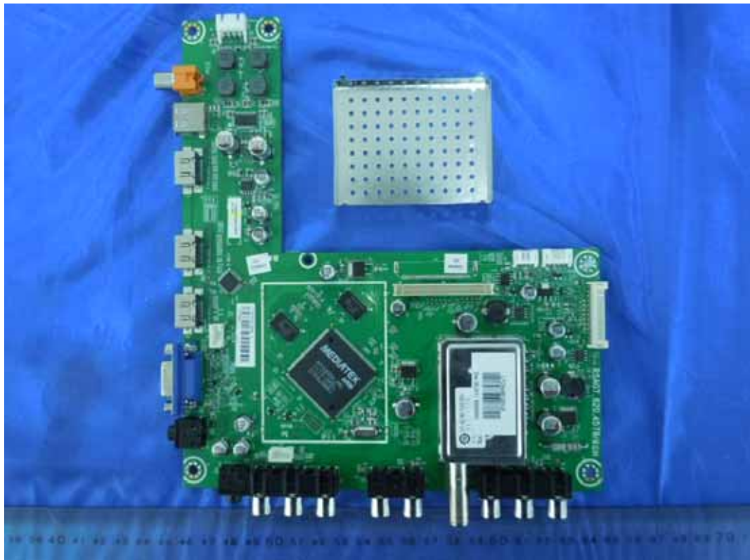
FIGURE 4 LED LCD TV (M/N: LTDN46K20US) MAIN BOARD (COMPONENT SIDE)
