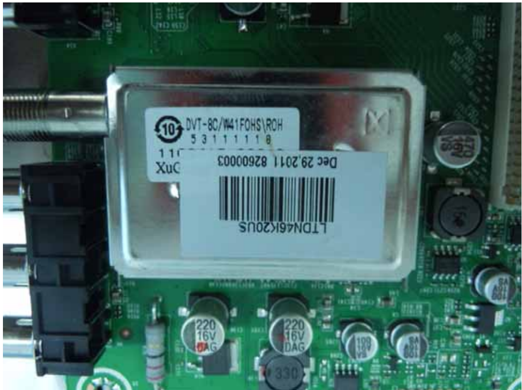
FIGURE 6 LED LCD TV (M/N: LTDN46K20US) TUNER ON MAIN BOARD
