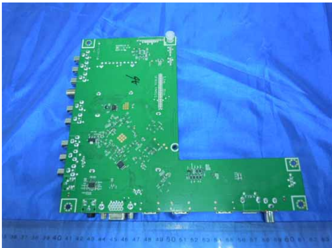
FIGURE 5 LED LCD TV (M/N: LTDN46K20US) MAIN BOARD (SOLDERED SIDE)
