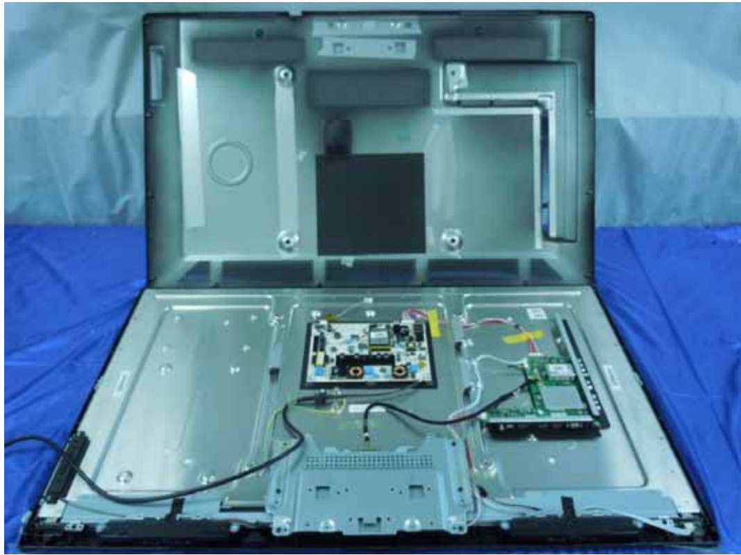
FIGURE 1 LED LCD TV (M/N: LTDN46K20US) COVER REMOVED
