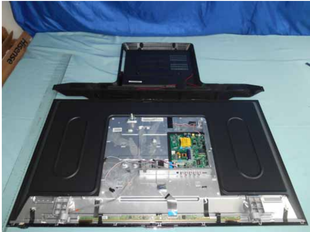
FIGURE 5 LED LCD TV (M/N: LC-40N3000U) COVER REMOVED
