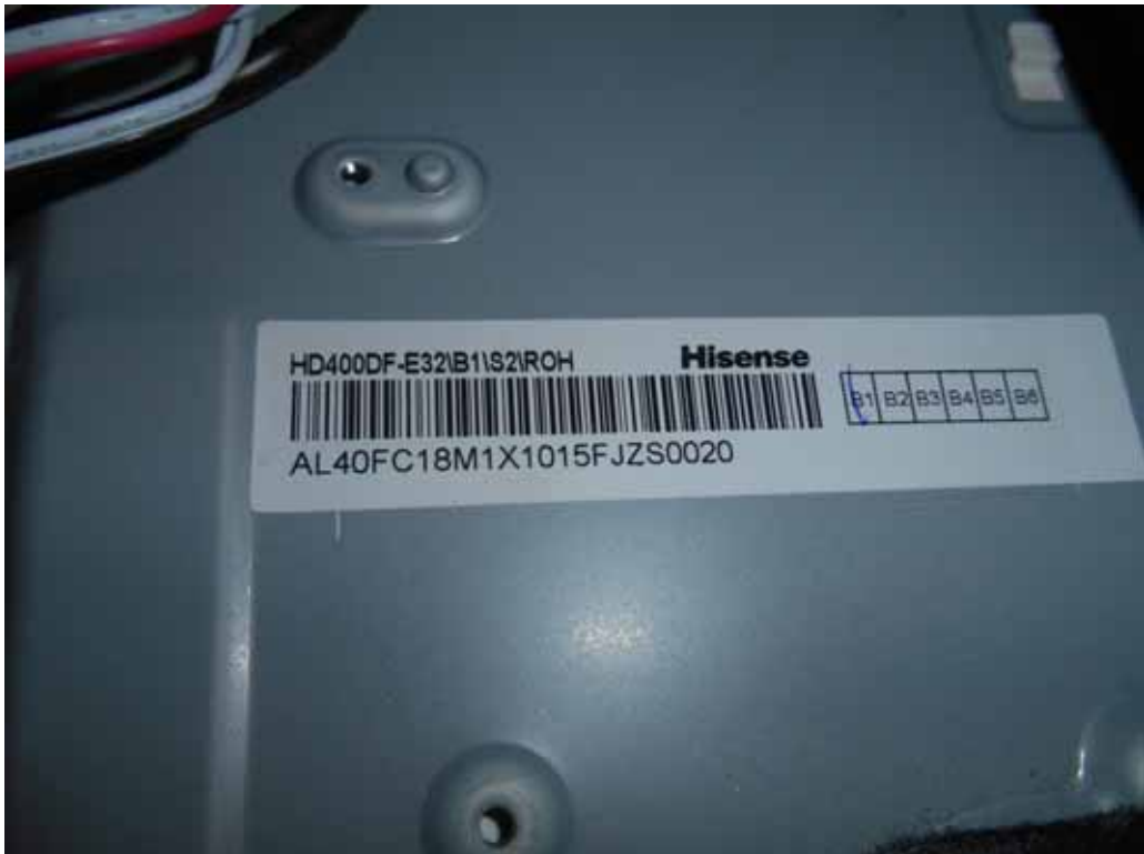
FIGURE 2 LED LCD TV (M/N: LTDN40K2207WUS) LCD PANEL LABEL
