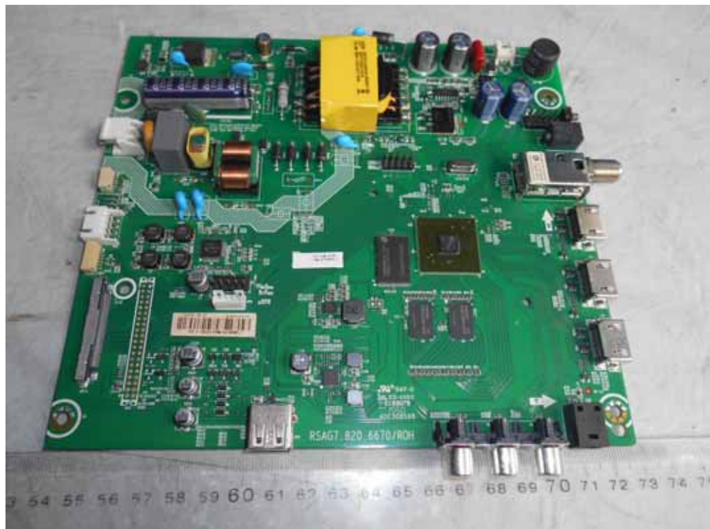
FIGURE 3 LED LCD TV (M/N: LTDN40K2207WUS) MAIN BOARD (COMPONENT SIDE)
