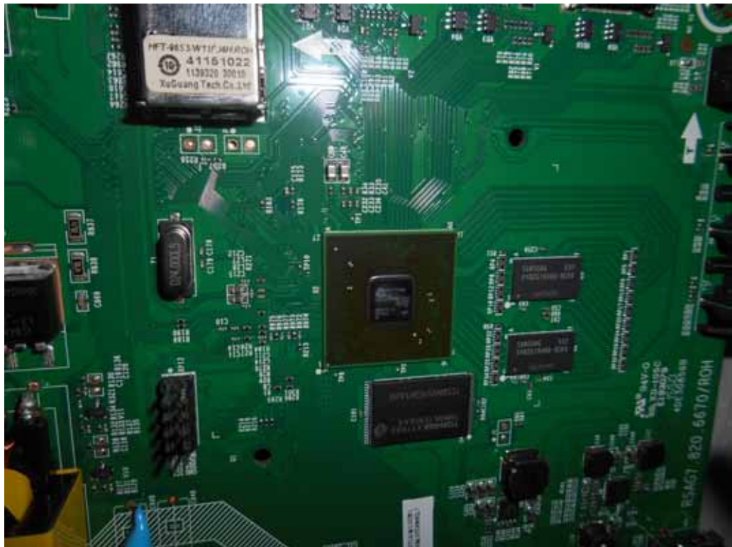
FIGURE 5 LED LCD TV (M/N: LTDN40K2207WUS) CHIP#1 & CRYSTAL#1 ON MAIN BOARD
