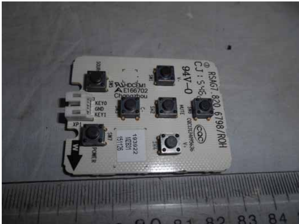
FIGURE 13 LED LCD TV (M/N: LTDN40K2207WUS) KEY BOARD (COMPONENT SIDE)
