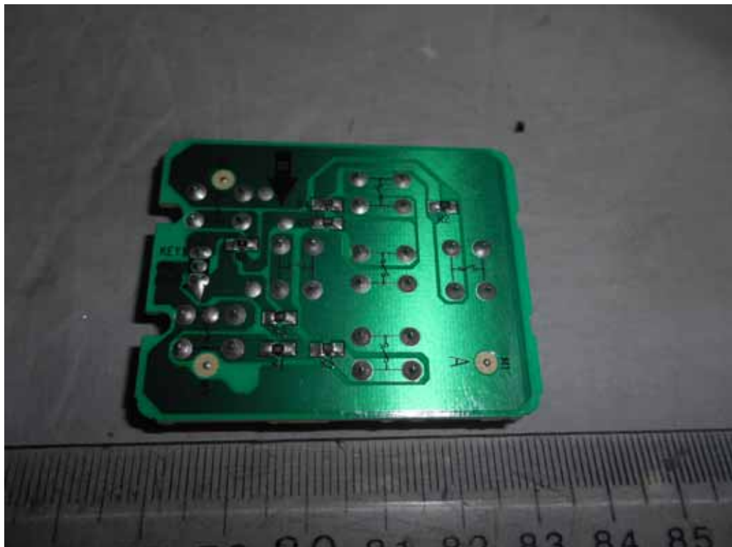
FIGURE 14 LED LCD TV (M/N: LTDN40K2207WUS) KEY BOARD (SOLDERED SIDE)
