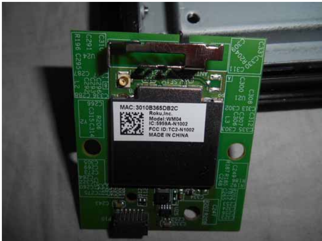
FIGURE 12 LED LCD TV (M/N: LTDN40K2207WUS) RF BOARD LABEL
