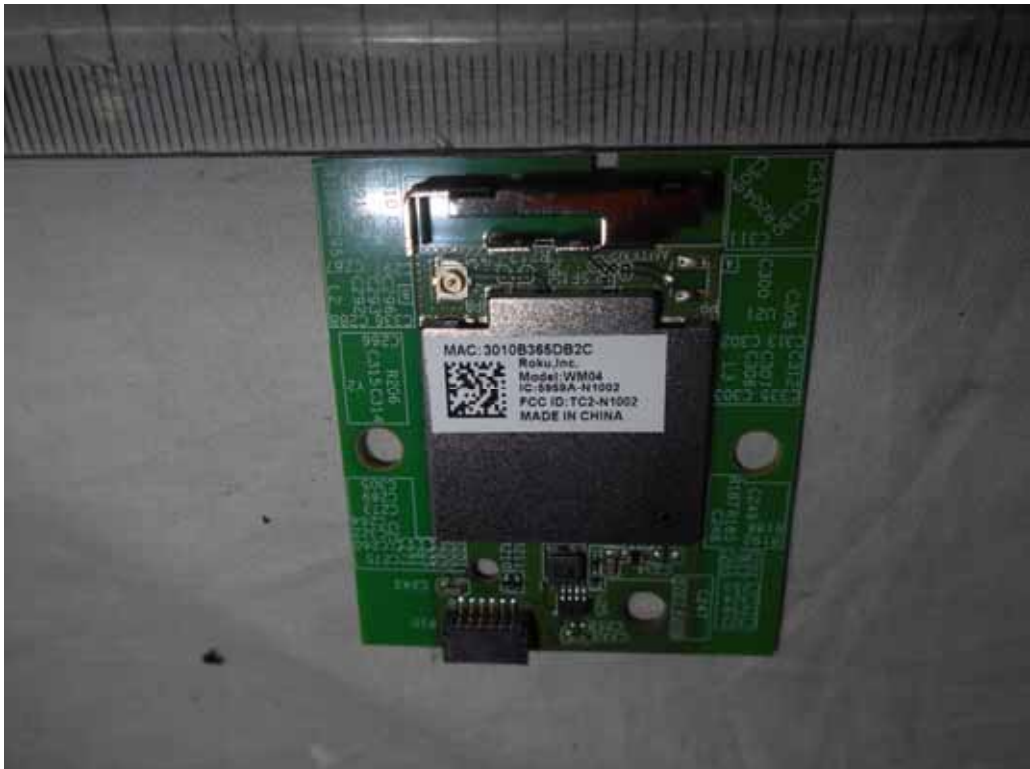
FIGURE 10 LED LCD TV (M/N: LTDN40K2207WUS) RF BOARD (COMPONENT SIDE)
