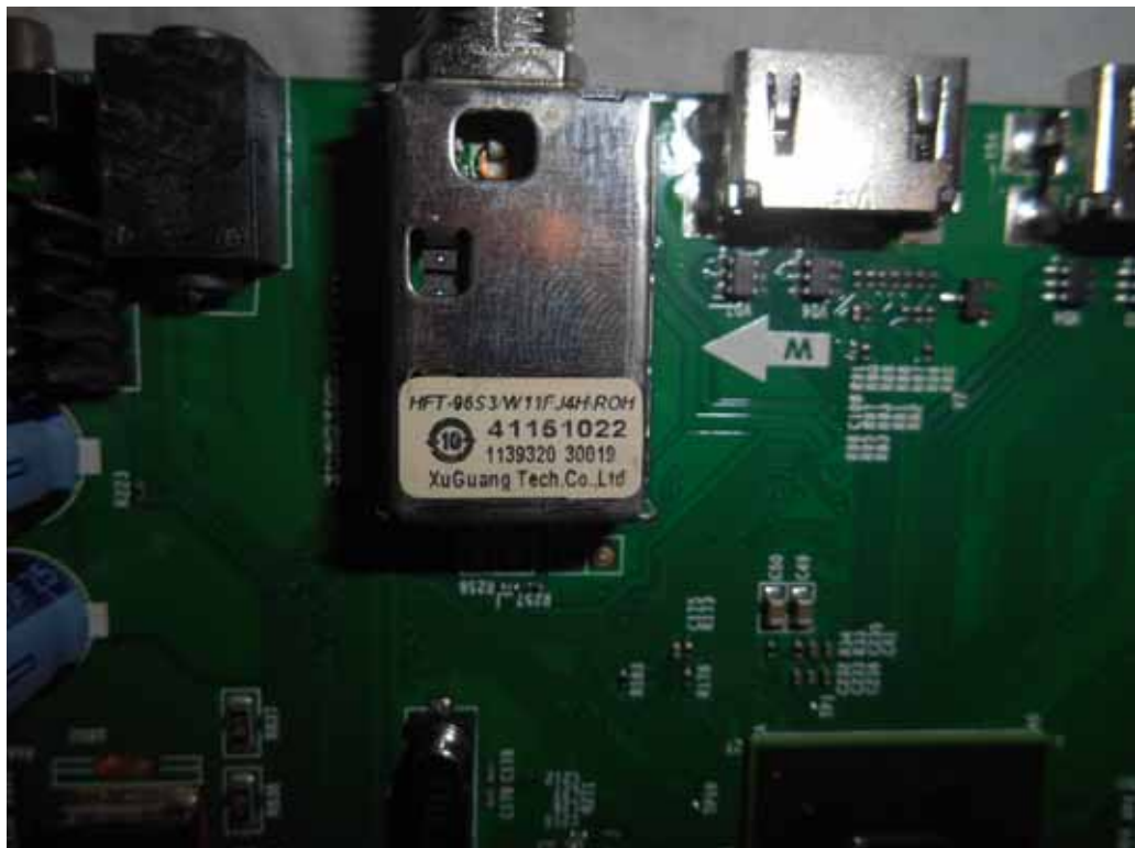
FIGURE 6 LED LCD TV (M/N: HU50K3300UWG) TUNER
