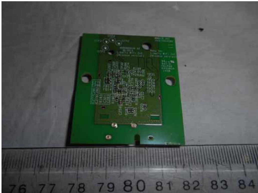
FIGURE 11 LED LCD TV (M/N: LTDN40K2207WUS) RF BOARD (SOLDERED SIDE)
