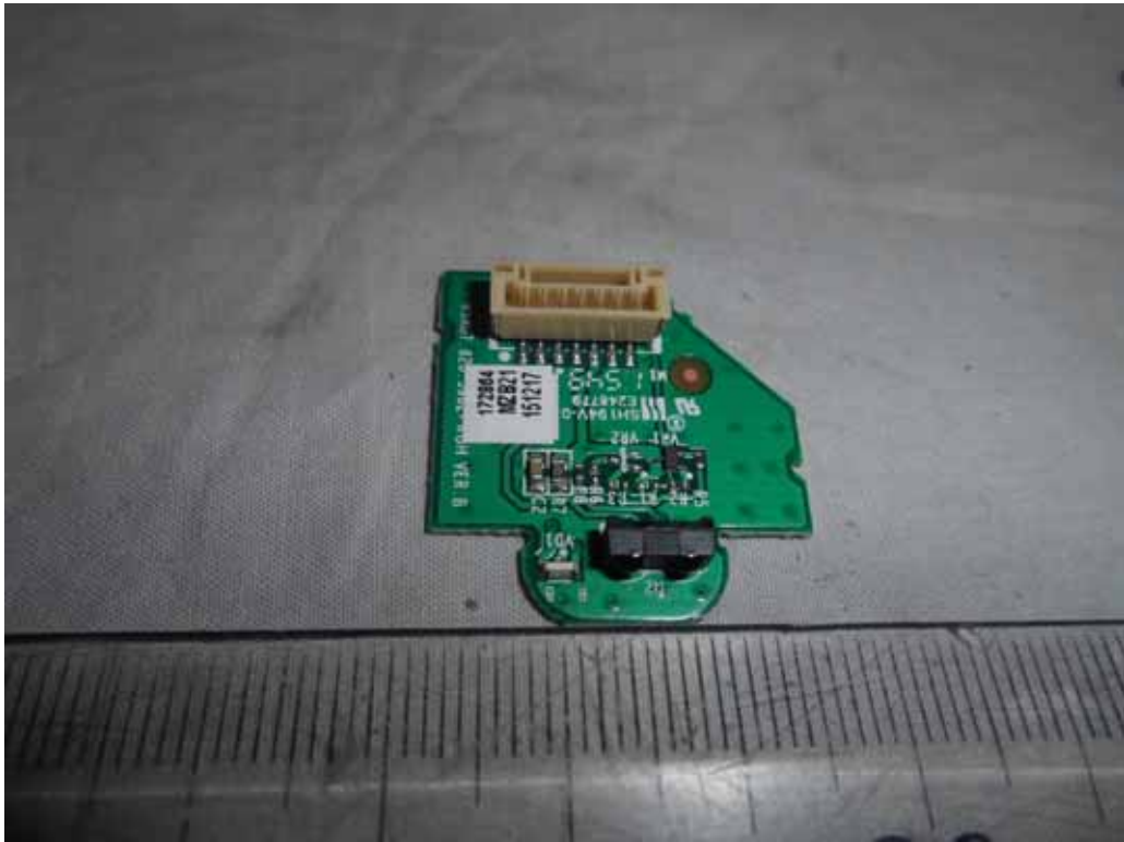
FIGURE 15 LED LCD TV (M/N: LTDN40K2207WUS) IR BOARD (COMPONENT SIDE)
