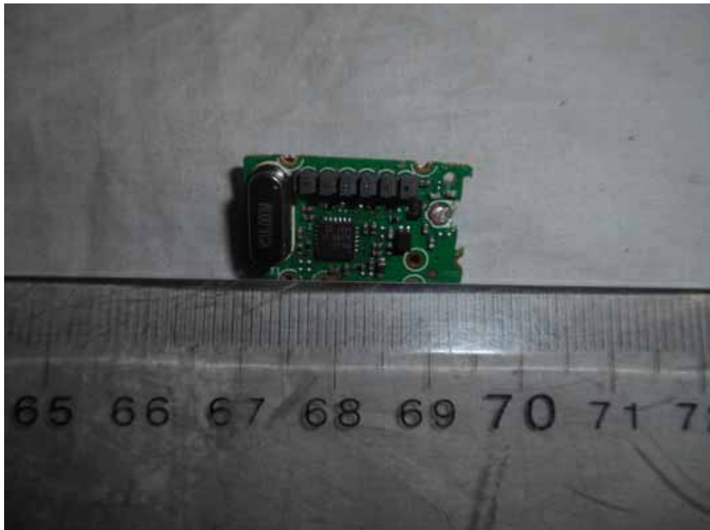
FIGURE 7 LED LCD TV (M/N: LTDN40K2207WUS) TUNER BOARD (COMPONENT SIDE)
