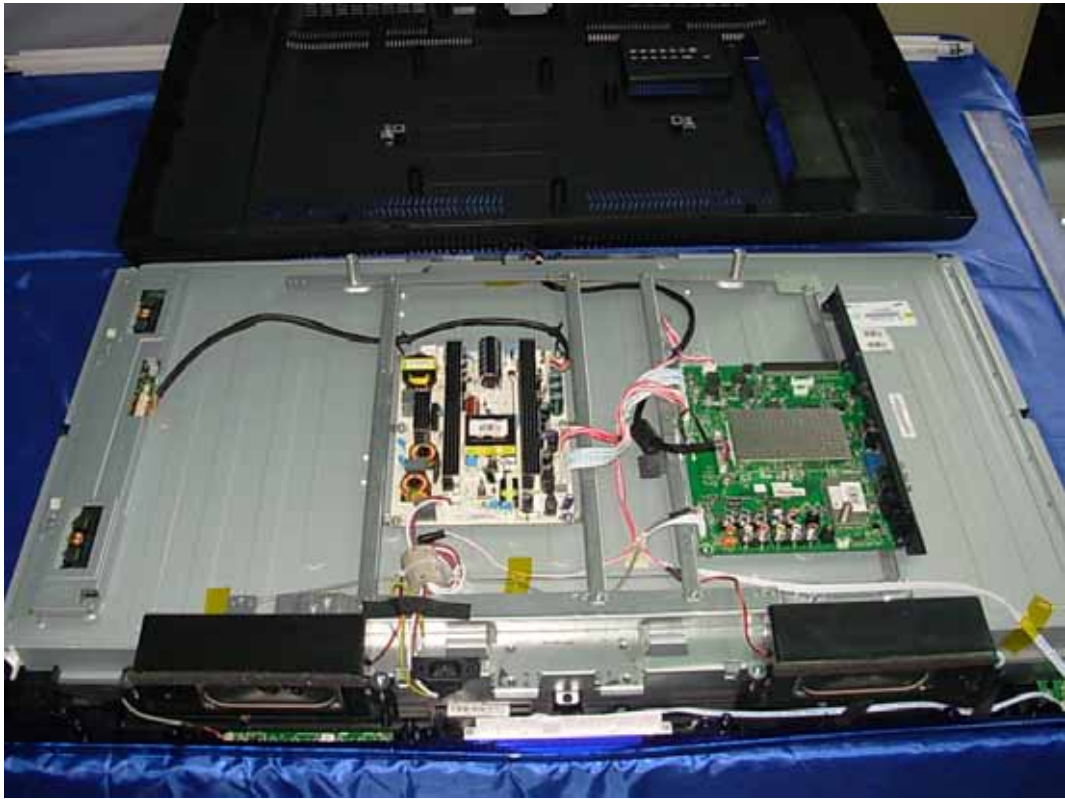
FIGURE 1 LCD TV (M/N: LTDN40V86MH) COVER REMOVED
