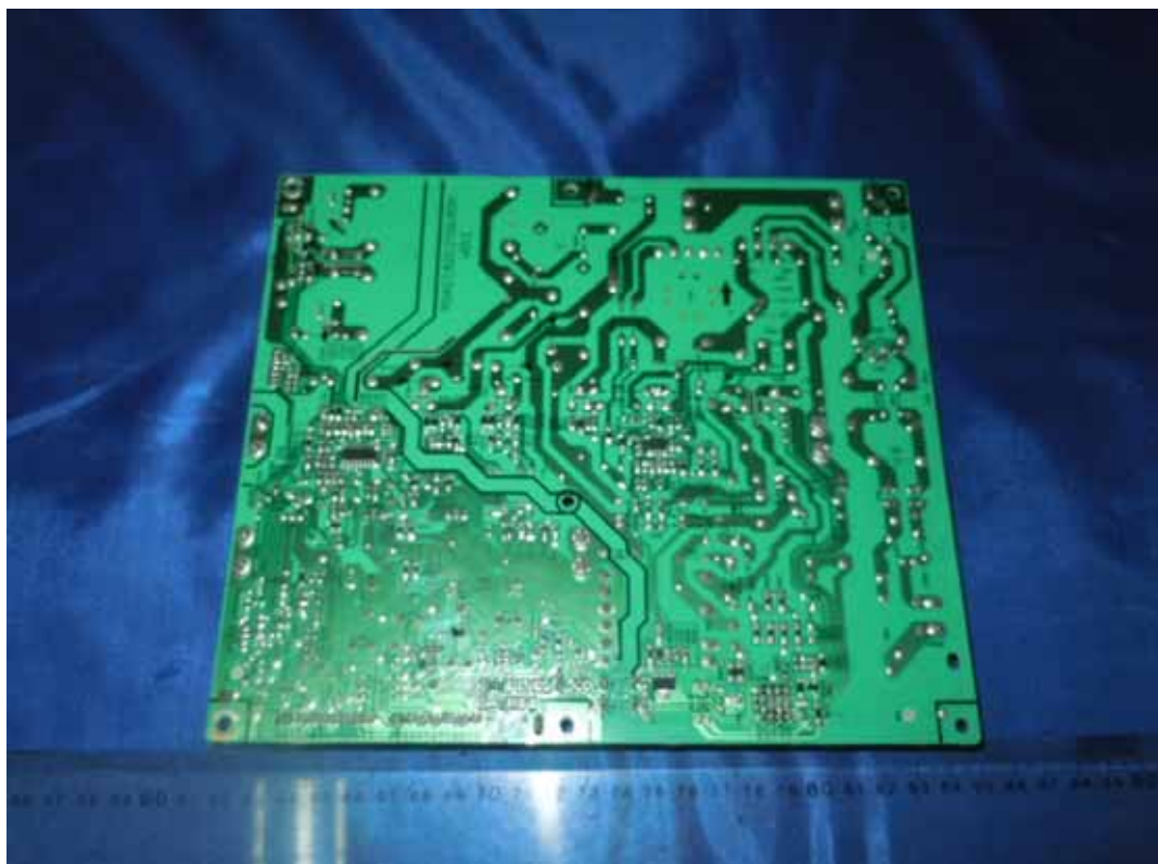
FIGURE 4 LCD TV (M/N: LTDN42V77US) POWER BOARD (SOLDERED SIDE)
