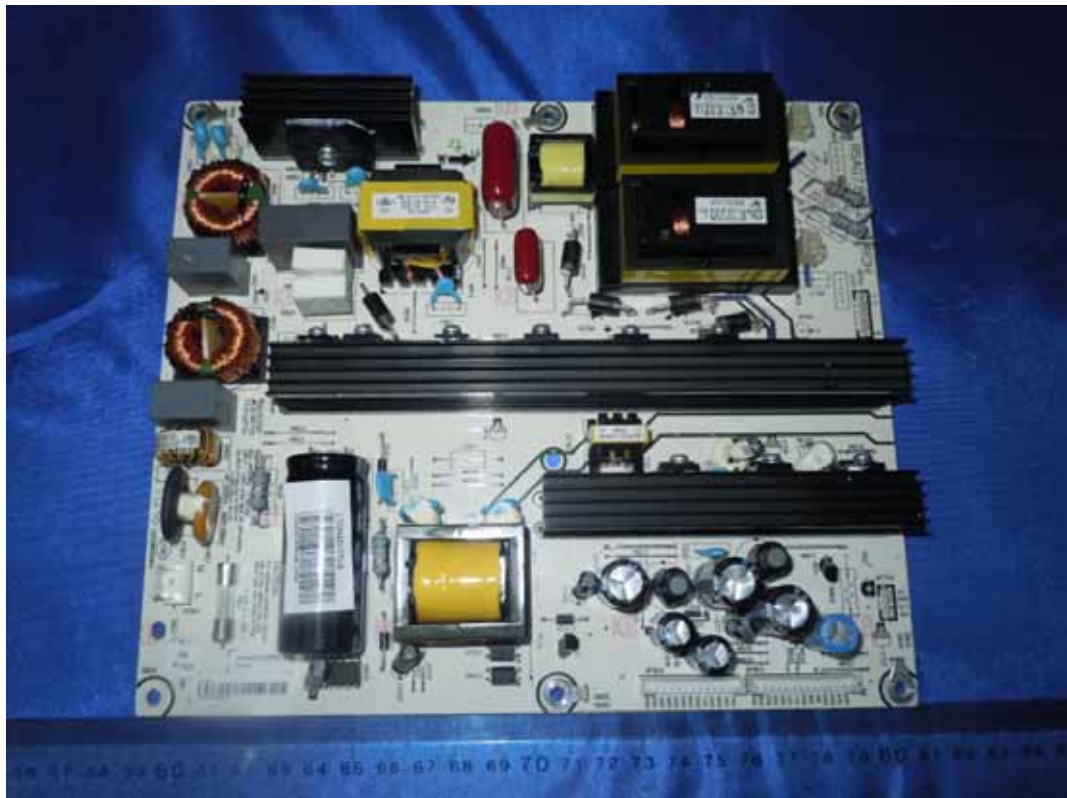
FIGURE 3 LCD TV (M/N: LTDN42V77US) POWER BOARD (COMPONENT SIDE)
