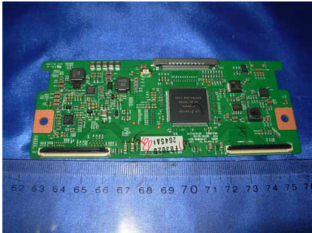
FIGURE 9 LCD TV (M/N: LTDN42V77US) CONTROL BOARD (COMPONENT SIDE)
