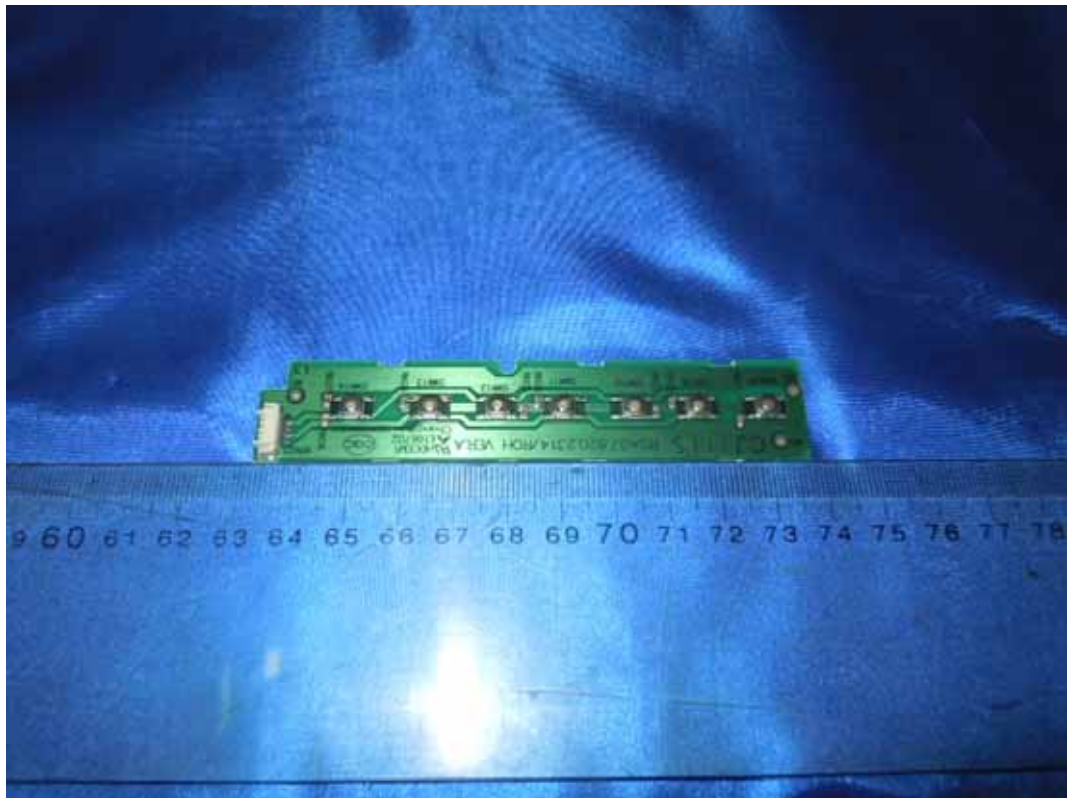
FIGURE 11 LCD TV (M/N: LTDN42V77US) KEY BOARD (COMPONENT SIDE)
