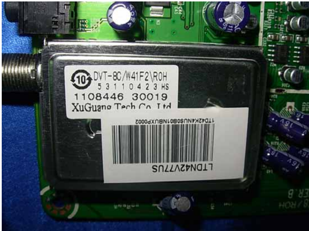
FIGURE 7 LCD TV (M/N: LTDN42V77US) TUNER ON MAIN BOARD
