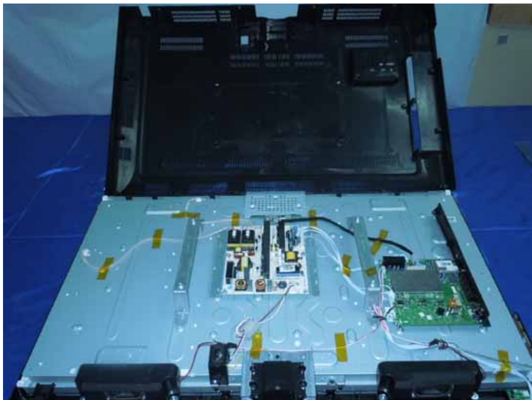
FIGURE 1 LCD TV (M/N: LTDN42V77US) COVER REMOVED
