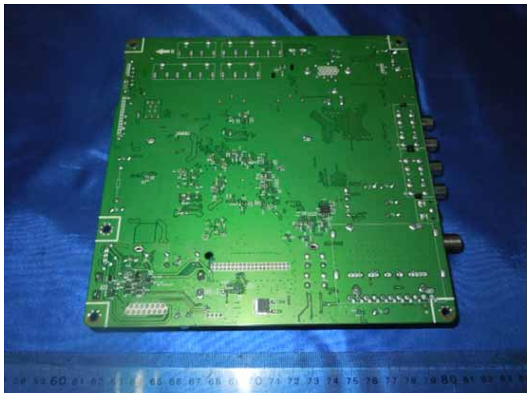
FIGURE 6 LCD TV (M/N: LTDN42V77US) MAIN BOARD (SOLDERED SIDE)
