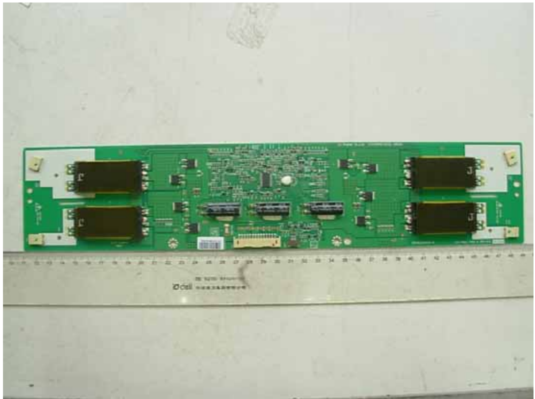
FIGURE 16 LCD TV (M/N: LTDN42V87XUS) HIGH VOLTAGE SIGNAL BOARD (COMPONENT SIDE)
