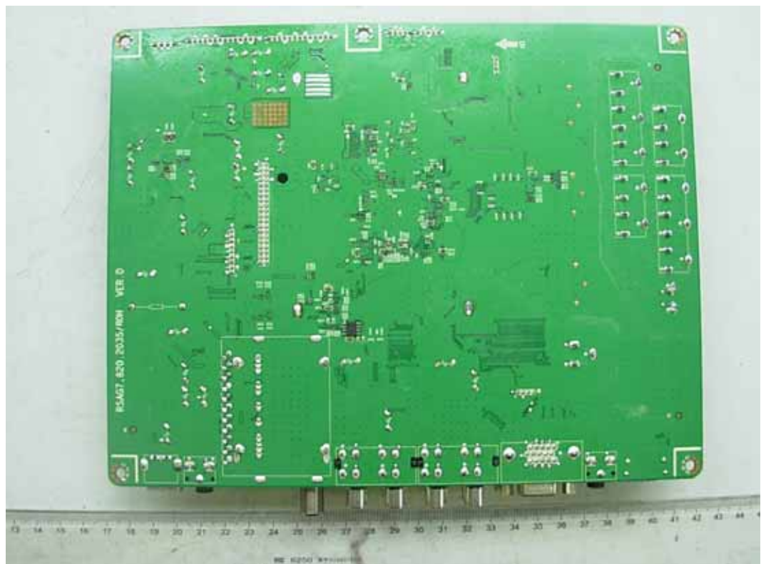
FIGURE 5 LCD TV (M/N: LTDN42V87XUS) MAIN BOARD (SOLDERED SIDE)
