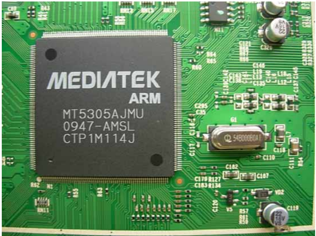
FIGURE 6 LCD TV (M/N: LTDN42V87XUS) CHIP #1 & CRYSTAL ON MAIN BOARD
