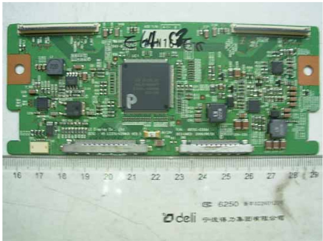
FIGURE 13 LCD TV (M/N: LTDN42V87XUS) LCD PANEL MAIN BOARD (COMPONENT SIDE)
