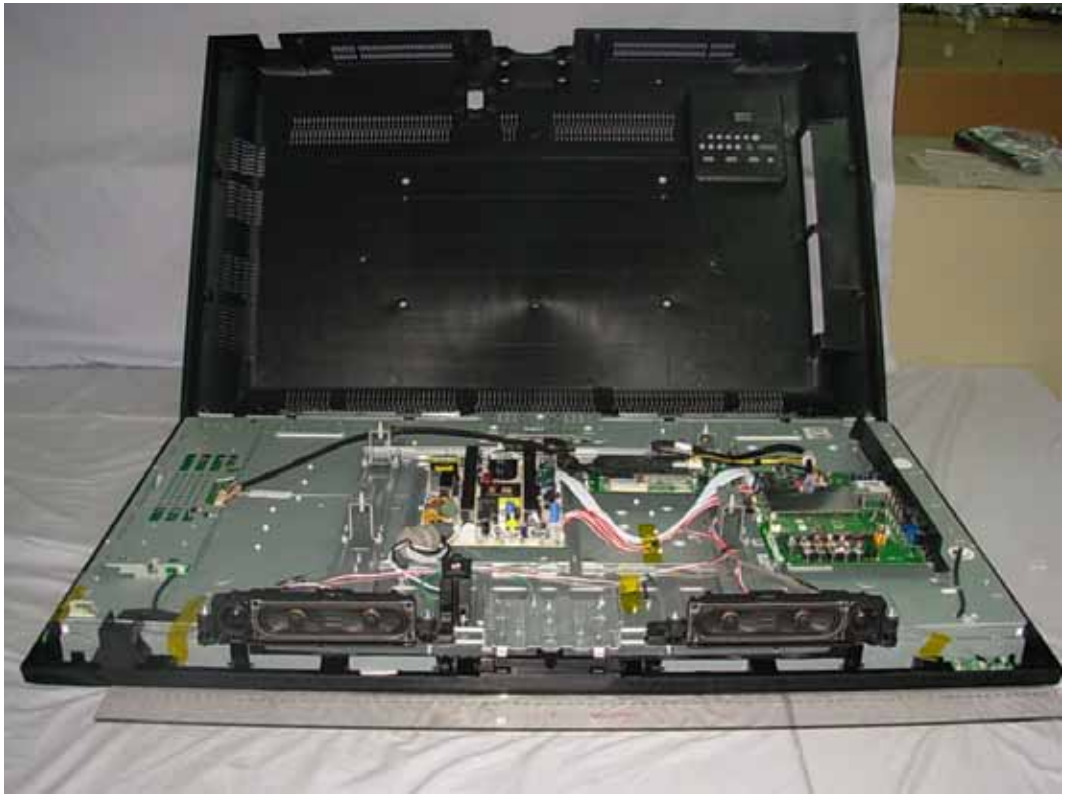
FIGURE 1 LCD TV (M/N: LTDN42V87XUS) COVER REMOVED
