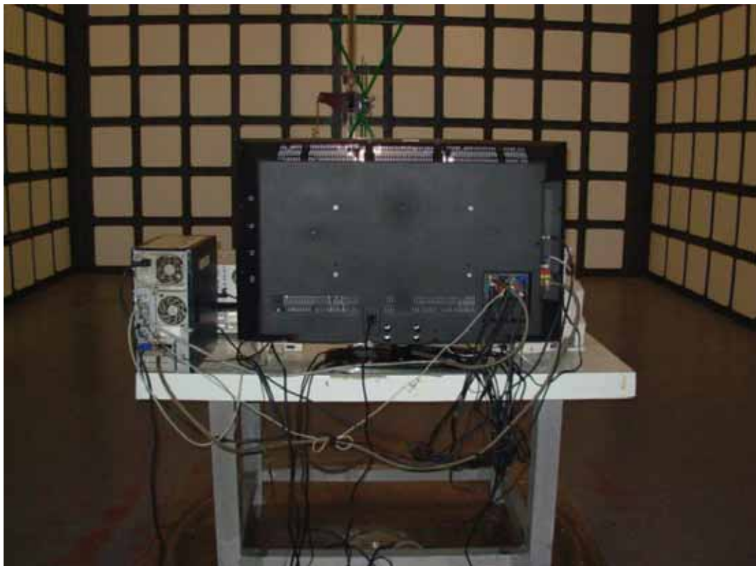
BACK VIEW OF RADIATED EMISSION TEST
