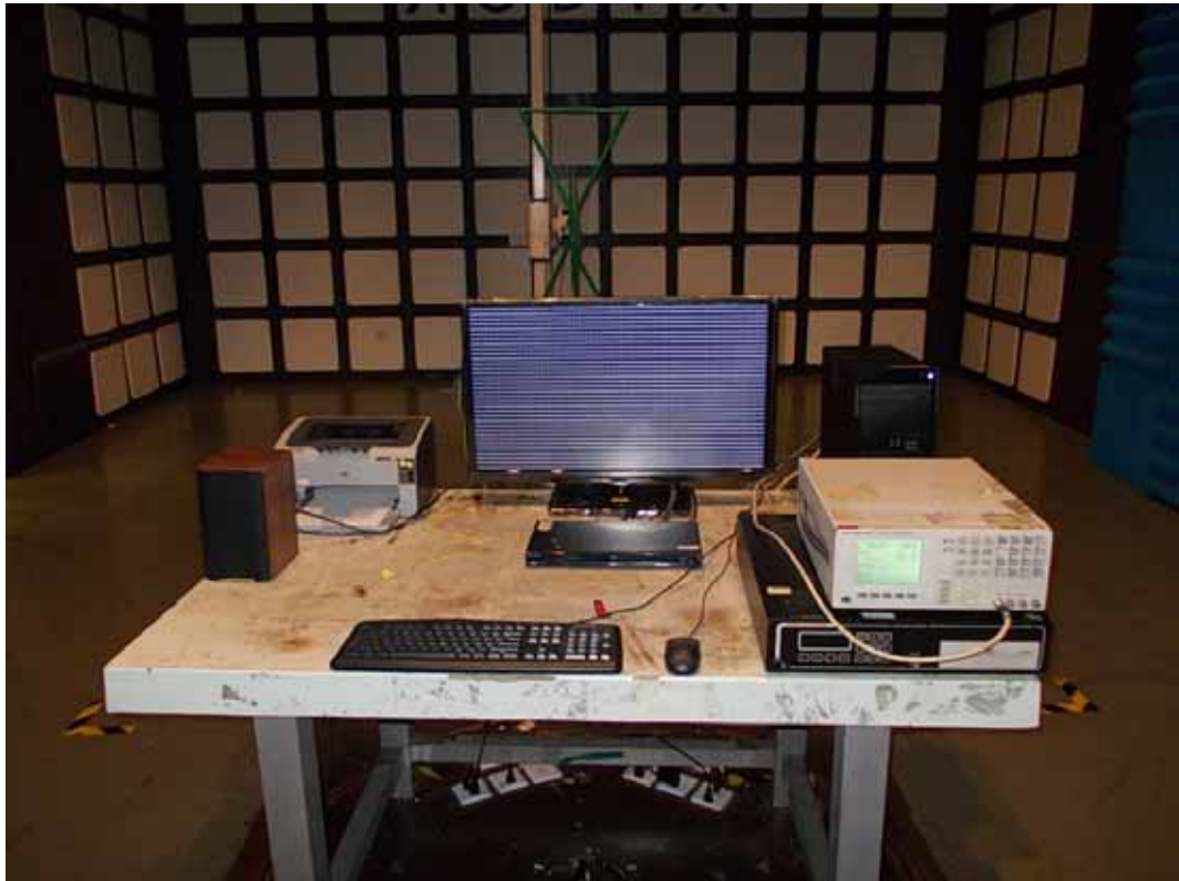
FRONT VIEW OF RADIATED EMISSION TEST
