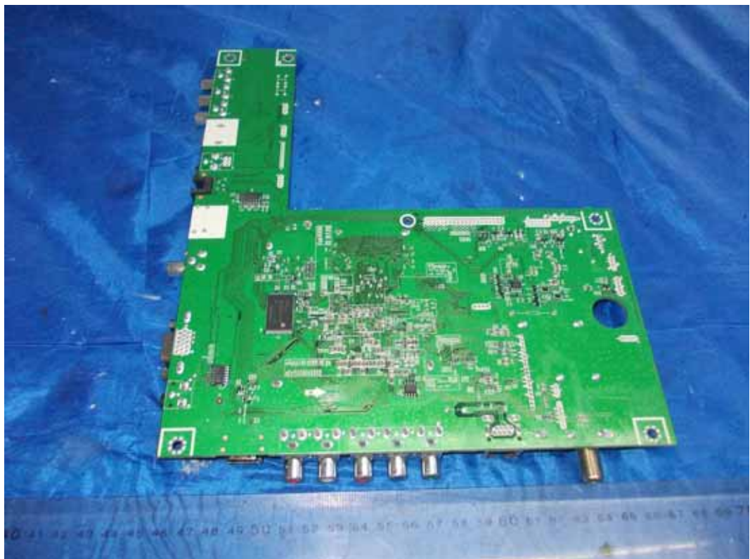
FIGURE 6 LED LCD TV (M/N: LHD32K366MH) MAIN BOARD (SOLDERED SIDE)
