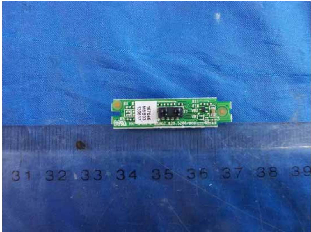
FIGURE 13 LED LCD TV (M/N: LHD32K366MH) IR BOARD (COMPONENT SIDE)
