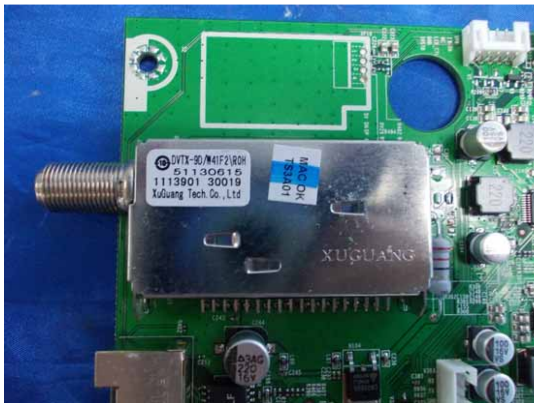
FIGURE 7 LED LCD TV (M/N: LHD32K366MH) TUNER ON MAIN BOARD
