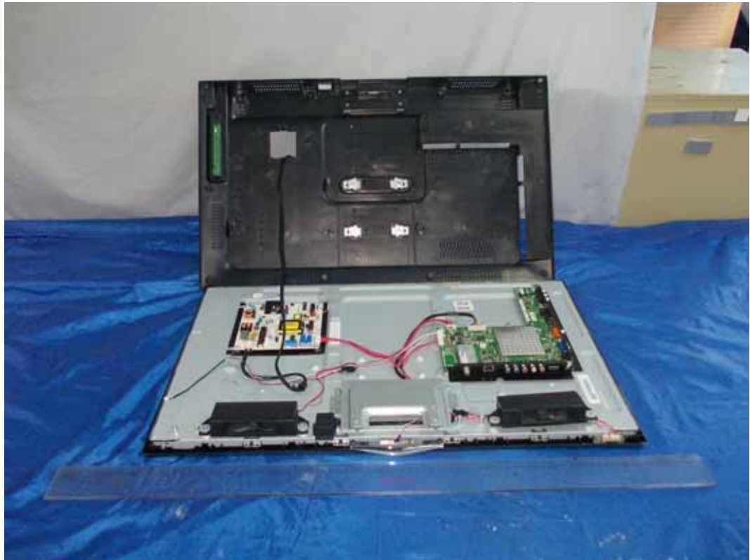
FIGURE 1 LED LCD TV (M/N: LHD32K366MH) COVER REMOVED
