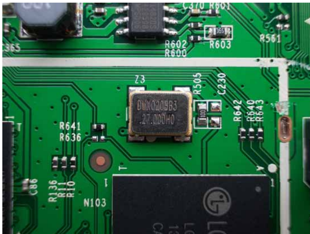
FIGURE 10 LED LCD TV (M/N: LHD32K366MH) CHIP & CRYSTAL ON MAIN BOARD
