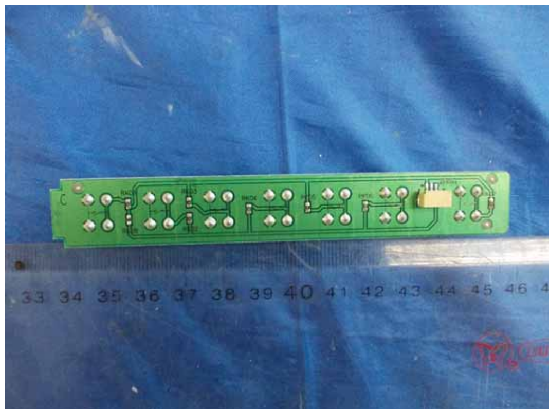
FIGURE 12 LED LCD TV (M/N: LHD32K366MH) KEY BOARD (SOLDERED SIDE)
