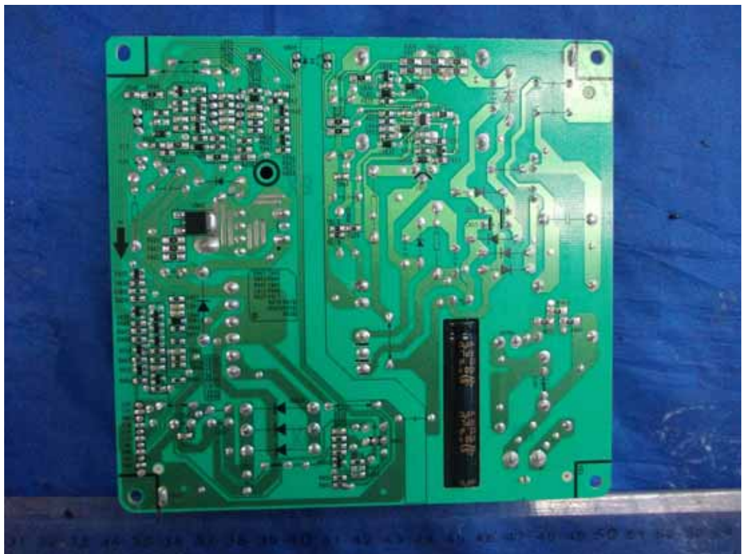
FIGURE 4 LED LCD TV (M/N: LHD32K366MH) POWER BOARD (SOLDERED SIDE)
