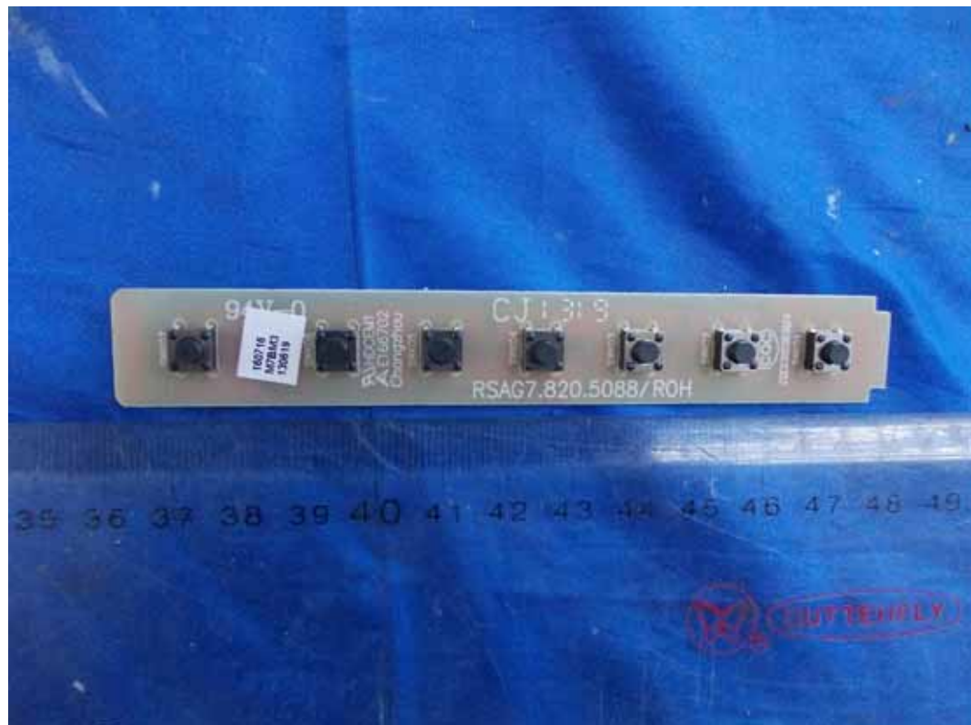
FIGURE 11 LED LCD TV (M/N: LHD32K366MH) KEY BOARD (COMPONENT SIDE)
