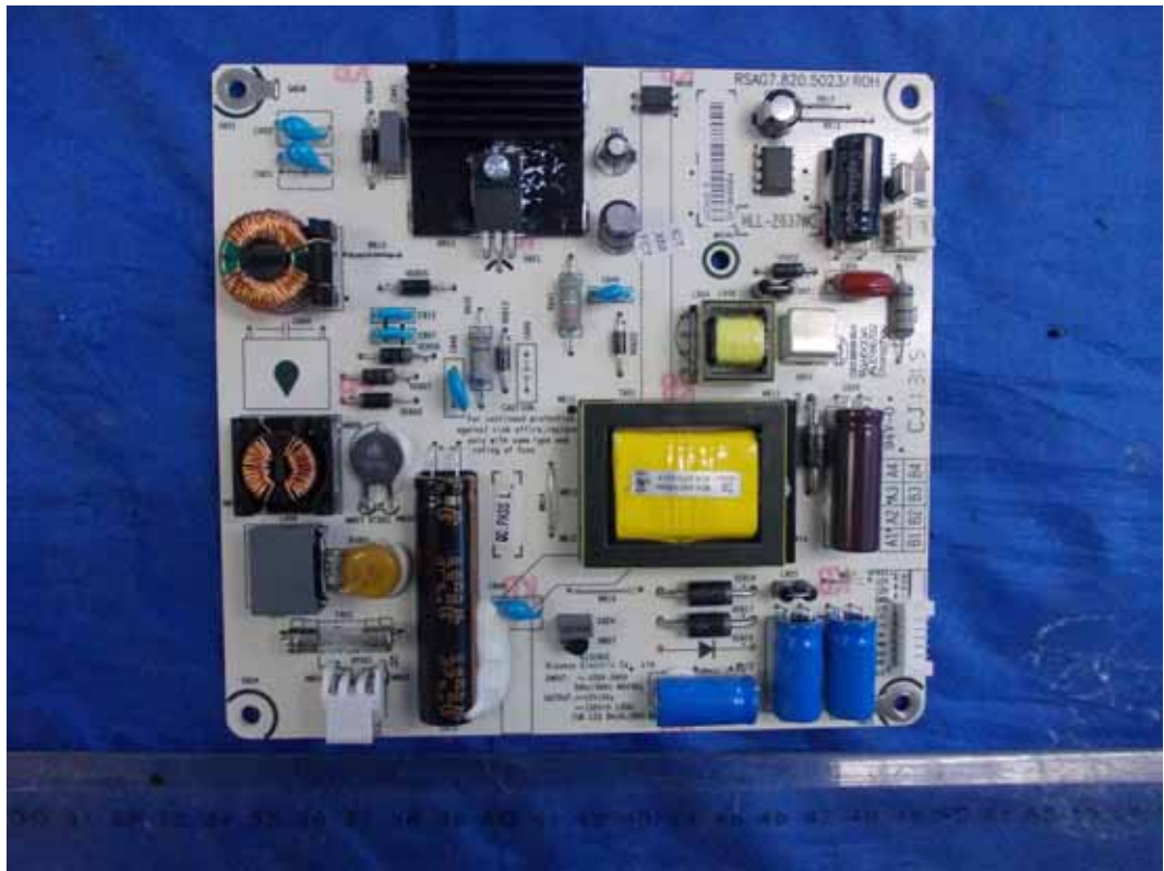
FIGURE 3 LED LCD TV (M/N: LHD32K366MH) POWER BOARD (COMPONENT SIDE)
