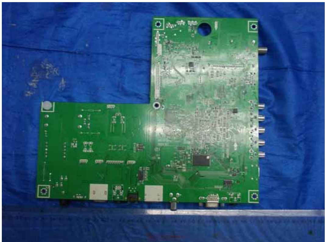
FIGURE 6 LED LCD TV (M/N: LHD32K366HS) MAIN BOARD (SOLDERED SIDE)
