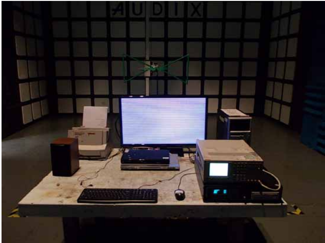
FRONT VIEW OF RADIATED EMISSION TEST
