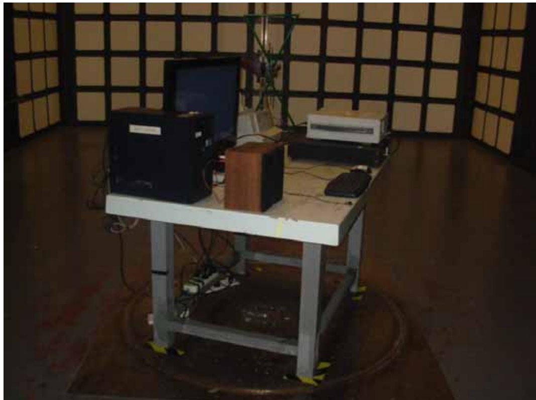
SETUP WITH MAXIMUM DETECTED EMISSION AT VERTICAL POLARIZATION (D-SUB 800*600@60Hz )
