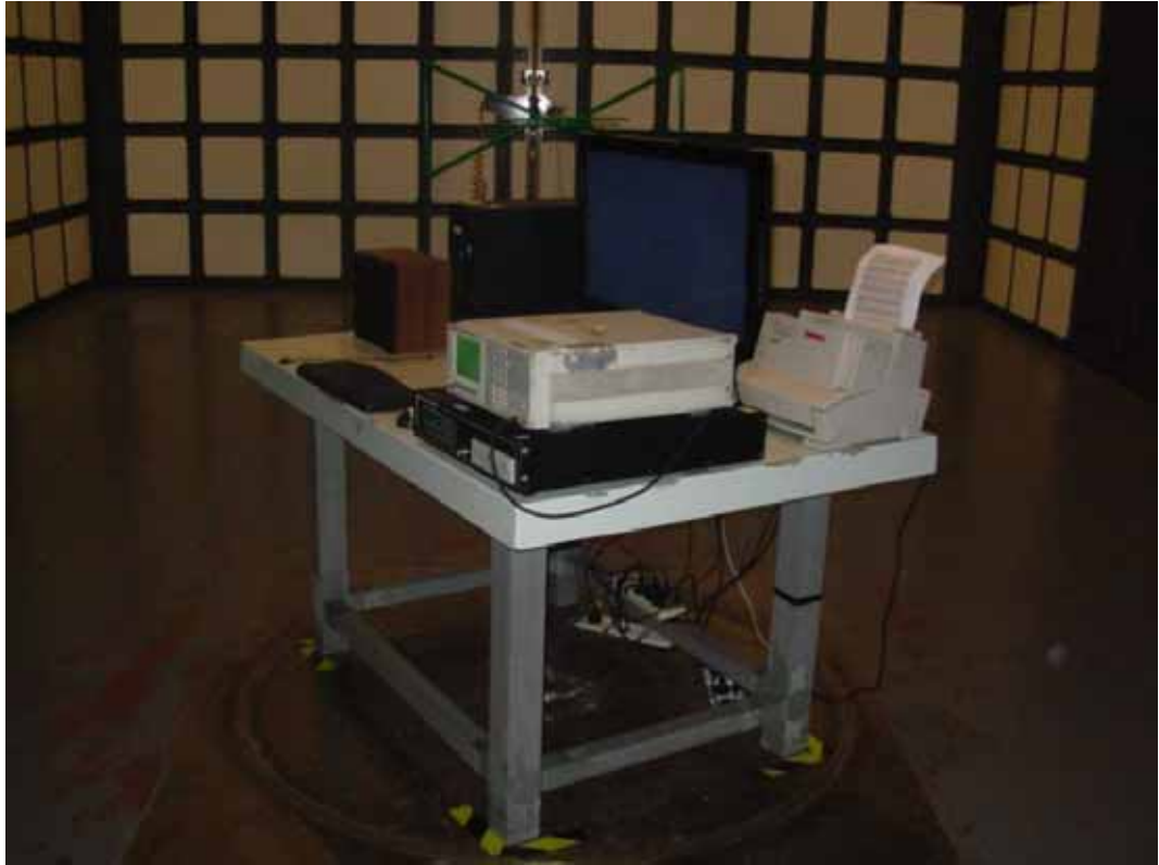
SETUP WITH MAXIMUM DETECTED EMISSION AT HORIZONTAL POLARIZATION (D-SUB 800*600@60Hz)
