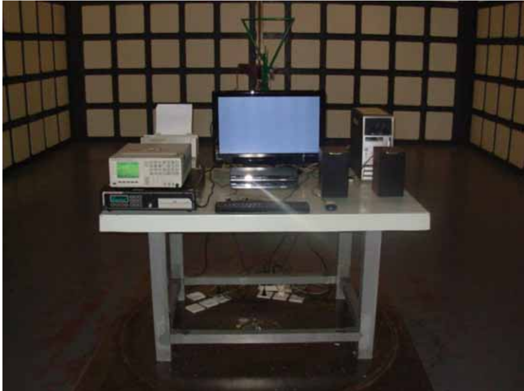
FRONT VIEW OF RADIATED EMISSION TEST
