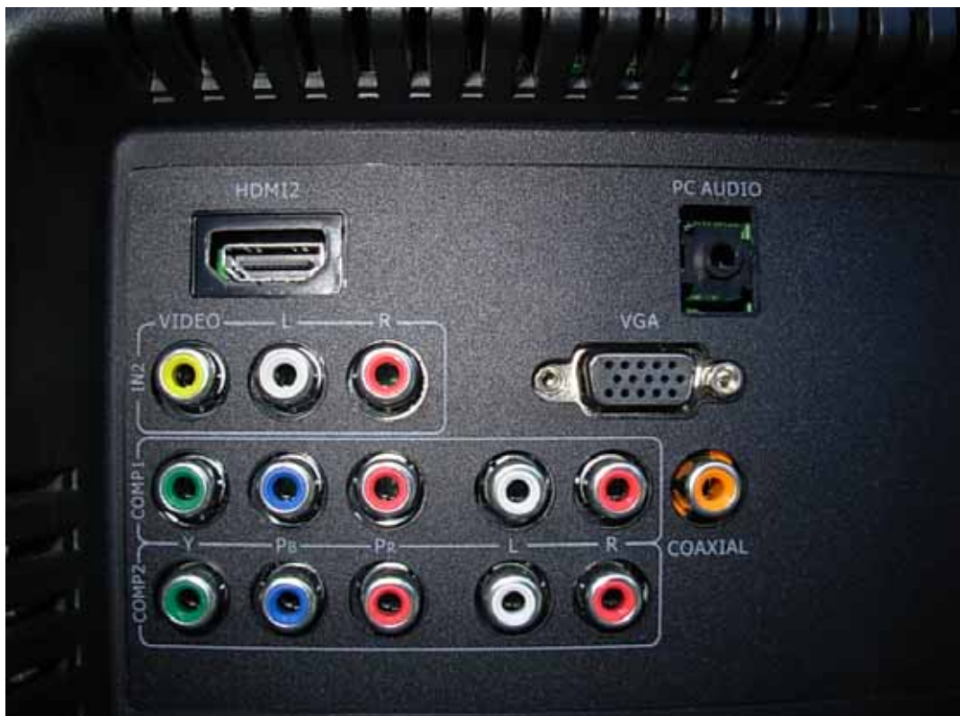
FIGURE 4 LCD TV (M/N: LCD32W57KCA) SIGNAL PORTS 1
