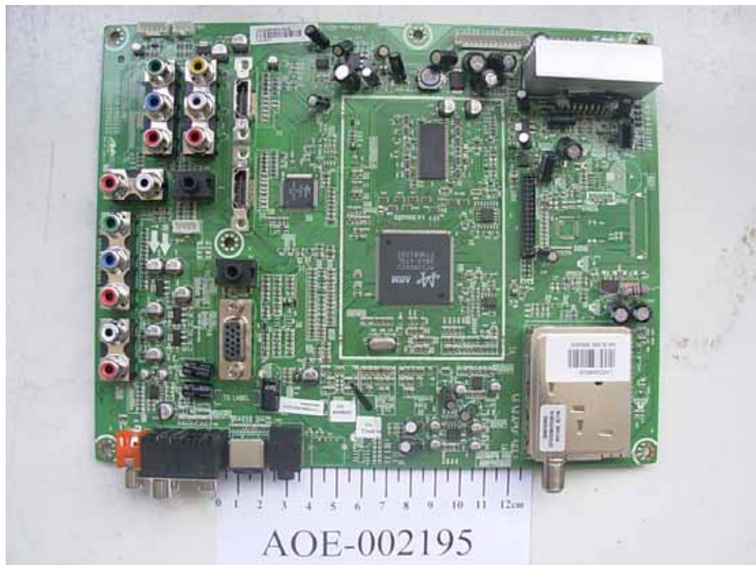
FIGURE 4 LCD TV (M/N: LHD32W57US) MAIN BOARD (COMPONENT SIDE)
