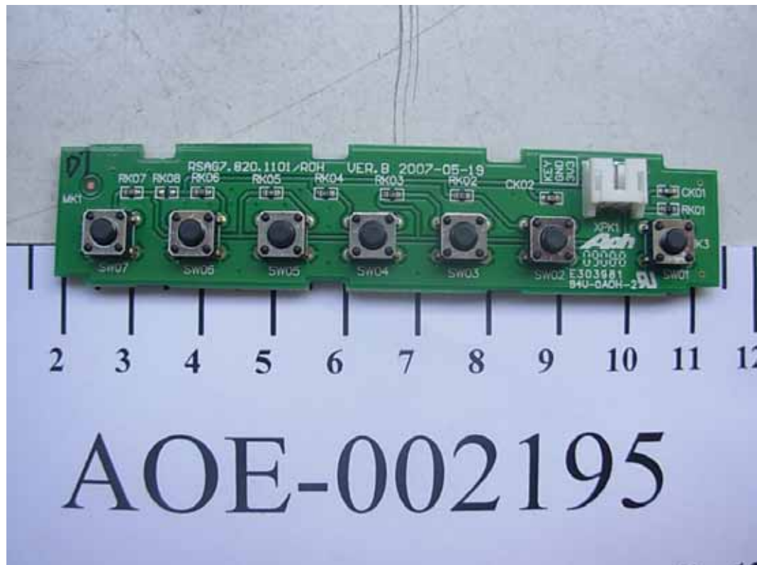
FIGURE 11 LCD TV (M/N: LHD32W57US) BUTTON BOARD (COMPONENT SIDE)
