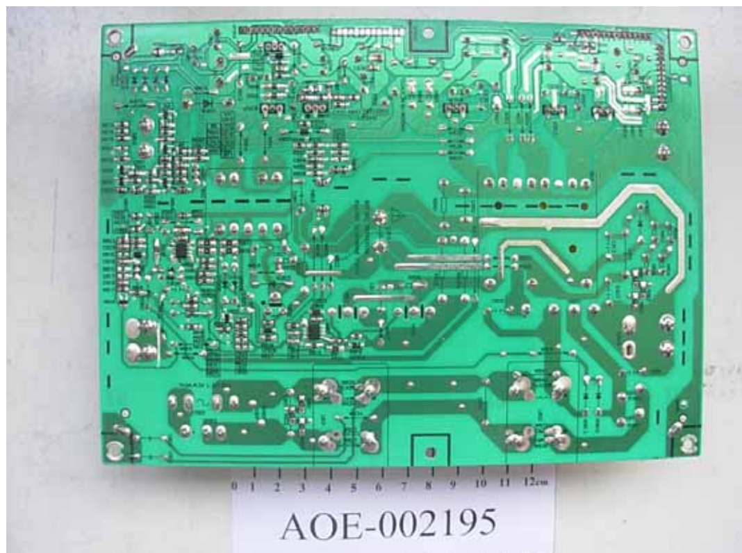
FIGURE 3 LCD TV (M/N: LHD32W57US) POWER BOARD (SOLDERED SIDE)
