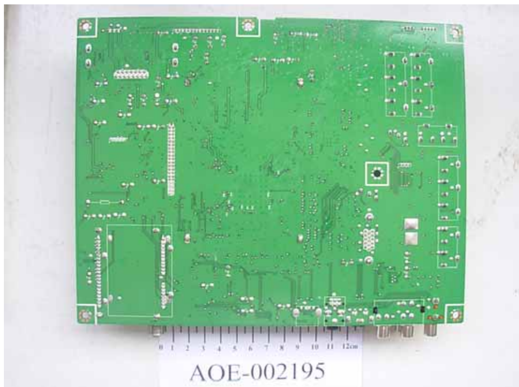
FIGURE 5 LCD TV (M/N: LHD32W57US) MAIN BOARD (SOLDERED SIDE)
